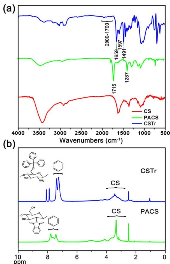
**Figure 1.** (a) FTIR spectra of CS, PACS and CSTr; (b) <sup>1</sup>H NMR spectra of PACS and CSTr.
