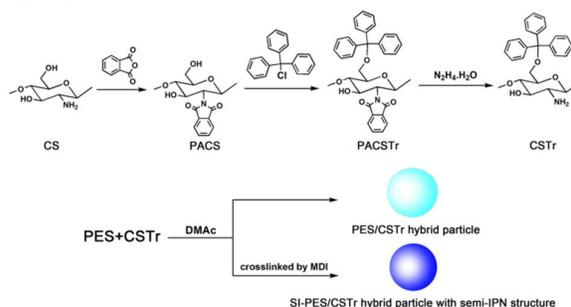
**Scheme 1.** The schematic illustration for preparing PES/CS, PES/CSTr and SI-PES/CSTr particles using Method 1 and Method 2, respectively.
