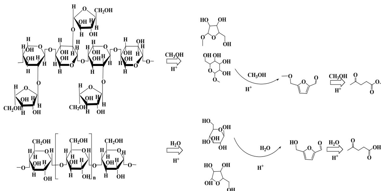
Fig. 8 Catalytic conversion of bamboo in methanol and in water medium.
