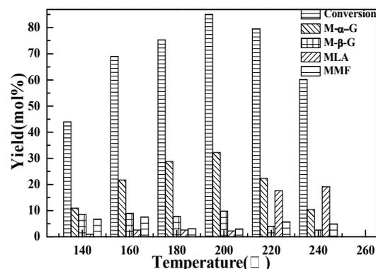
**Fig. 4** Effect of reaction temperature on the conversion of bamboo.
