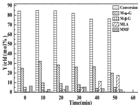
**Fig. 3** Effect of reaction time on the conversion of bamboo; Reaction conditions: temperature, 200 °C; catalyst, 0.8 g; bamboo, 40 g; methanol, 350 mL. M- $\alpha$ -G, methyl- $\alpha$ -glucoside; M- $\beta$ -G, methyl- $\beta$ -glucoside; MLA, methyl levulinate; MMF, 5-methoxymethyl furfural (MLG include M- $\alpha$ -G and M- $\beta$ -G; yields based on HPLC and GC analysis).
