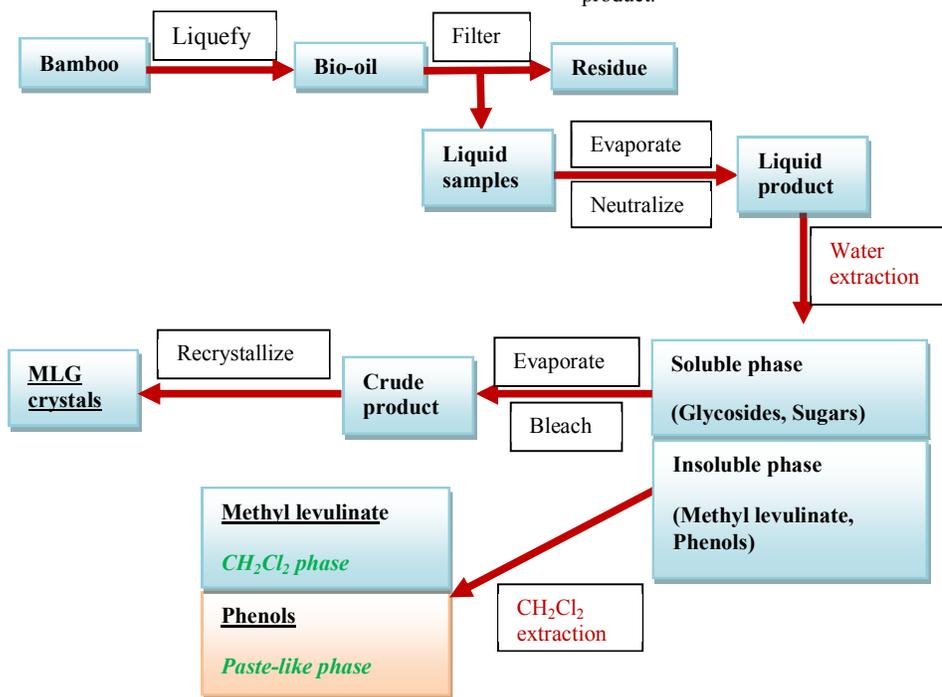
Scheme 1 The production and separation of MLG via the extraction from liquefied product.
