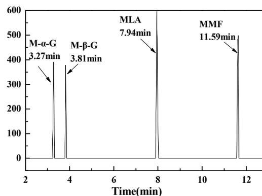
**Fig. 1** The HPLC analysis of standard M- $\alpha$ -G, M- $\beta$ -G, MLA, and MMF.
