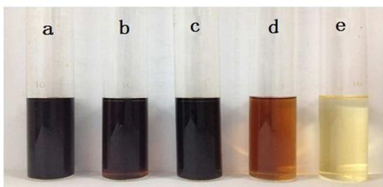
**Fig. 2** Effect of different agents on liquefied product bleaching. (a) liquefied product, (b)  $\text{H}_2\text{O}_2$ , (c)  $\text{NaHSO}_3$ , (d)  $\text{O}_3$ , and (e) activated carbon.
