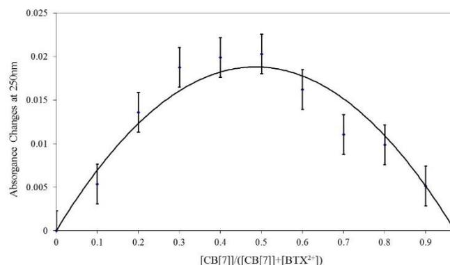
**Fig. 3.** Job's plot indicating 1:1 host-guest complex stoichiometry for {BTX·CB[7]}<sup>2+</sup> complex based on the continuous variation UV-visible titration monitored at 250 nm.
