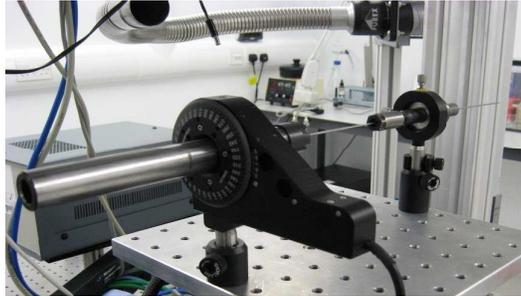
**Figure 1** Stent on mandrel held together by two collets (one in a rotary stage) on an XYZ stage.
