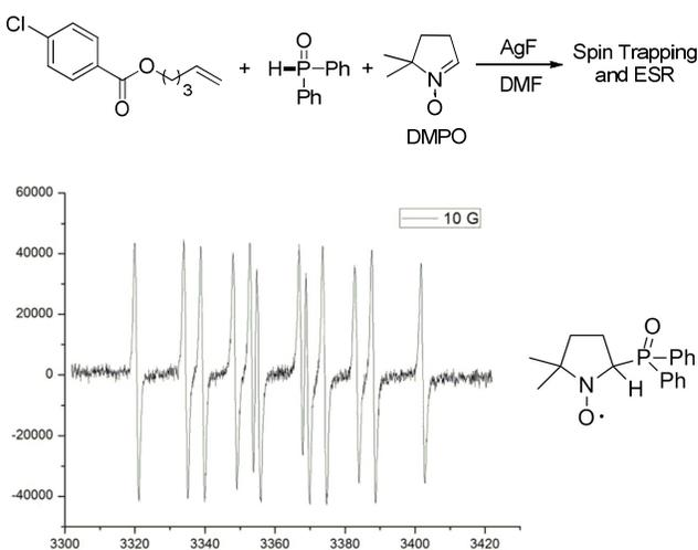
**Scheme 4.** ESR studies. ESR spectrum of a solution of pent-4-en-1-yl 4-chlorobenzoate ( $5.0 \times 10^{-2} \text{ mol/L}$ ), diphenylphosphine oxide (0.2 mol/L), AgF ( $1.0 \times 10^{-2} \text{ mol/L}$ ), and DMPO ( $6.0 \times 10^{-2} \text{ mol/L}$ ) in DMF (2 mL), 110 °C for 2.5 h.
