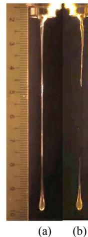
**Fig. 5** Extrusion of the 10% w/v alginate solution through a nozzle at 80°C (a) before droplet breakup and (b) after droplet breakup. Heat loss from the droplets when they were extruded. The droplets were dropped into the gelling bath.
