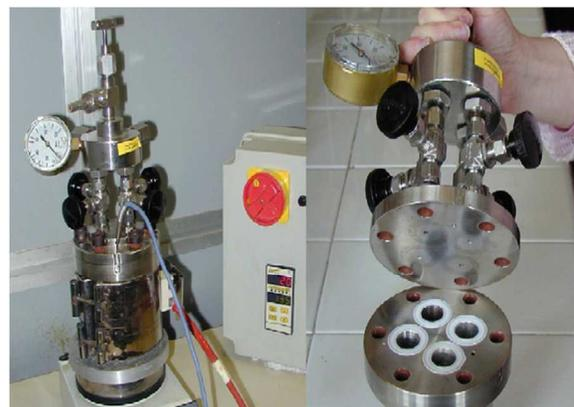
Fig. 2 4x-parallel stainless steel autoclave
