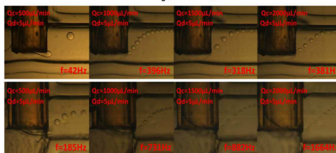
Figure 3 (Color online) Droplet formation frequencies under different conditions. Droplet formation frequencies are extracted from the image analysis of the high speed video. Formation frequencies in the step channel go larger with the increase of continuous phase flow rates. However, the frequencies in the straight channel decrease when continuous flow rates become higher, illustrated by the arise of widening jetting regime induced by the different flow fields.
