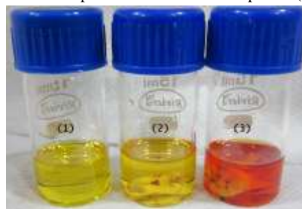
Fig. 4 Colorimetric detection of \text{F}^- from fluorosis affected tooth sample: (1) 1 \times 10^{-4} M DMSO solution of L ; (2) L remains silent with non fluorosis tooth sample; (3) after dipping the fluorosis affected tooth sample into the DMSO solution of L for 5 minutes.
