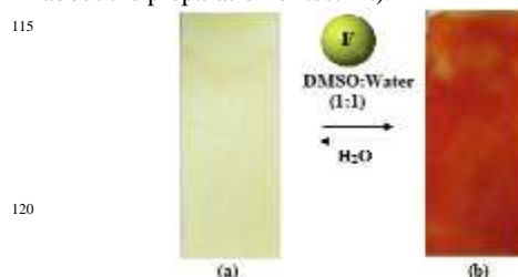
Fig. 10 Test kit (a) L coated test paper (b) \text{F}^- solution sprayed on L coated test paper.
