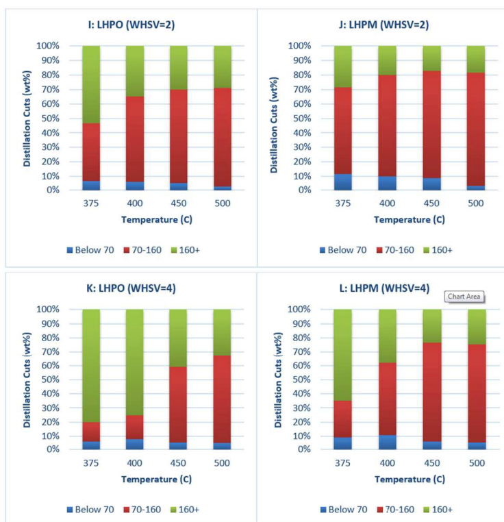
FIGURE 8: COMPARISON OF LHPO AND LHPM DISTILLATION CUTS (I-L)
