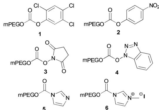
**Figure 1:** Common activated mPEG derivatives used for PEGylation of proteins by formation of urethane bonds. **1**: mPEG-trichlorophenyl carbonate (mPEG-TCP); **2**: mPEG-*p*-nitrophenyl carbonate (mPEG-pNPC); **3**: mPEG-succinimidyl carbonate (mPEG-SC); **4**: mPEG-benzotriazolyl carbonate (mPEG-BTC); **5**: mPEG-carbonylimidazole (mPEG-Im); **6**: mPEG-carbonylimidazolium iodide (mPEG-Im<sup>+</sup>I).
