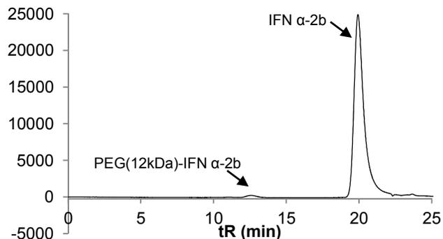
**Figure 2:** SE-HPLC analysis at 280 nm of PEGylation reaction mixture IFN- $\alpha$ 2b with reagent **5**, after 48 h of reaction.
