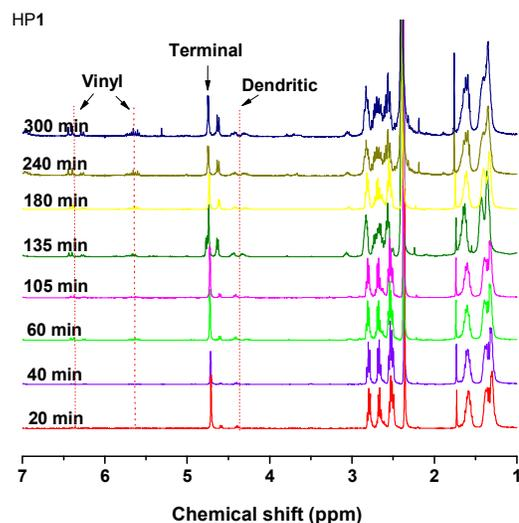
Fig. 3  $^1H$  NMR spectra of HP1 at different reactive time.
