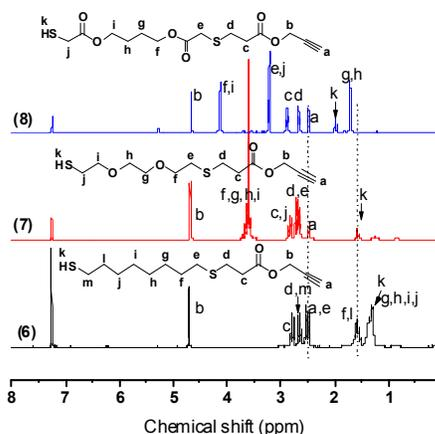
Fig. 1  $^1H$  NMR spectra of intermediates **6-8**.
