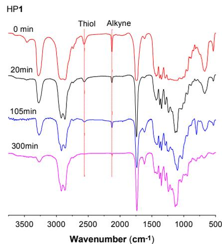
Fig. 4 FTIR spectra of HP1 at different reactive time.
