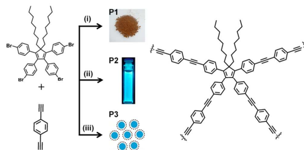
Scheme 1 Fabrication of porous organic polymers involving TBDC (tetrakis-(4-bromophenyl)-5,5-dioctylcyclopentadiene) and DEB (diethynyl benzene) in the form of powder (P1), soluble in organic solvents (P2) and aqueous dispersion of nanoparticles (P3). Fabrication conditions: (i) [Pd(PPh 3 ) 4 ], CuI, diisopropylamine, toluene, 80°C, 48 h, (ii) [Pd(PPh 3 ) 2 Cl 2 ], CuI, diisopropylamine, toluene, 80°C, 12 h and (iii) [Pd(PPh 3 ) 4 ], CuI, SDS, water, diisopropylamine, toluene, 50°C, 48 h.
