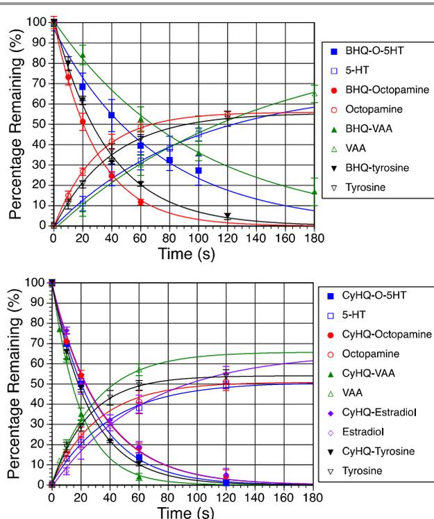
**Figure 4** Time courses for the photolysis of the photoactivatable phenols at 365 nm (IPE) and the rise of the biologically active phenols. Top: BHQ series, Bottom: CyHQ series. The percentage remaining is the average of at least 3 runs, and the error bars represent the standard deviation of the measurement. Lines are least-squares fits of a single exponential decay or a single exponential rise to max.
