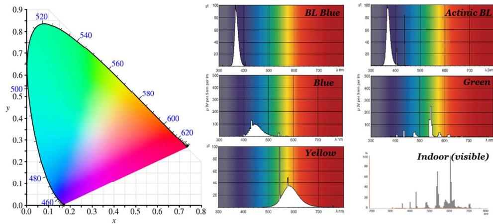
Figure 1 – International Commission on Illumination (CIE) color space chromaticity diagram and emission spectra of the fluorescent lamps
