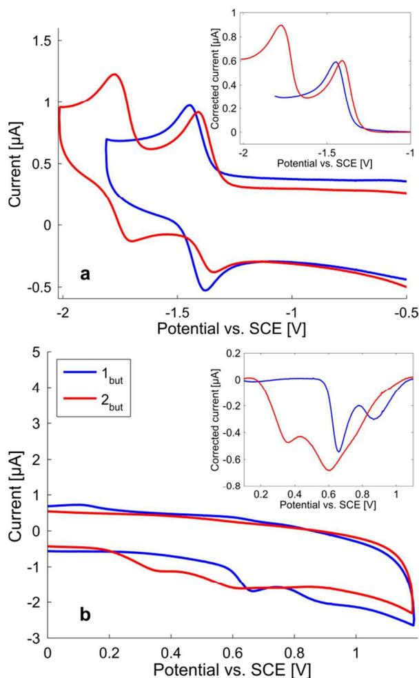
**Fig. 6.** Reduction (a) and oxidation (b) cyclic voltammograms for compounds  $\mathbf{1}_{\text{but}}$  (blue line) and  $\mathbf{2}_{\text{but}}$  (red line) recorded in dimethylformamide. The inserts show background-normalized
