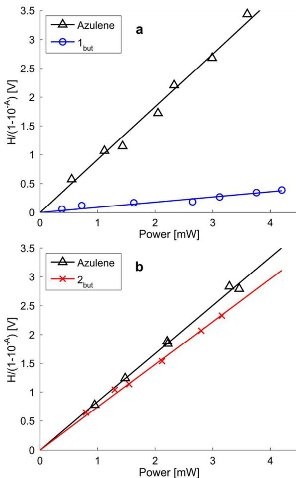
**Fig. 4.** Plots of the absorbance-corrected peak-to-peak amplitude of the initial LIOAC pressure wave against the incident laser power for nitrogen-saturated solutions of **1**<sub>but</sub> and **2**<sub>but</sub> along with the corresponding plot for the standard azulene. Linear fits to the data are shown.
