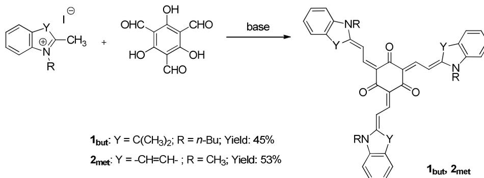
**Scheme 1.** Methodology used to synthesize **1<sub>but</sub>** and **2<sub>met</sub>**.
