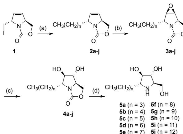
**Scheme 1.** Synthesis of  $\alpha$ -1-*C*-alkyl-DAB. Reagents: (a) alkylzinc bromide (3.2 eq.), Ni(cod)<sub>2</sub> (16 mol%), (*R,R*)-2,6-bis(4-isopropyl-2-oxazolin-2-yl)pyridine (32 mol%), *N,N*-dimethylacetamide, rt, 20 h (b) Oxone<sup>™</sup> (5.0 eq.), CF<sub>3</sub>COCH<sub>3</sub> (10.0 eq.), NaHCO<sub>3</sub> (7.5 eq.), 0 °C, 2 h (c) CF<sub>3</sub>CO<sub>2</sub>H (12.0 eq.), THF/H<sub>2</sub>O (3:2), reflux, 72 h (d) NaOH (10 eq.), EtOH/H<sub>2</sub>O (2:1), reflux, 1 h.
