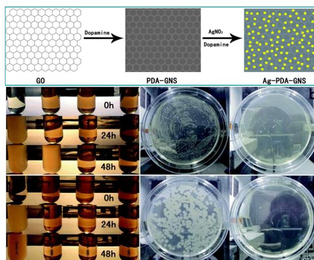
**Fig. 16** The top image shows the illustration of the procedure for preparing Ag-PDA-GNS. The bottom images are the antibacterial activities of Ag-PDA-GNS. LB liquid medium turbidity assays (a and c) and LB-agar plate tests (b and d) were employed to evaluate antibacterial activities toward Gram-negative bacteria *E. coli* cells (a and b) and Gram-positive bacteria *B. subtilis* (c and d). (reprinted with permission from Ref. <sup>235</sup>.)
