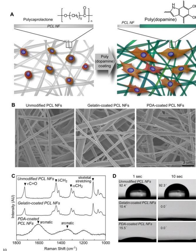
**Fig. 17** (A) Schematic illustration of cell adhesion on PDA-coated polycaprolactone nanofibers (PCL NFs). (B) SEM images, (C) Raman spectra, and (D) water contact angle measurement of unmodified, gelatin-coated, and PDA-coated PCL NFs. The increase of fiber diameter, new Raman peaks at 1350/1600  $\text{cm}^{-1}$ , and a decrease in the water contact angle indicate the formation of a PDA ad-layer on electrospun PCL NFs. (reprinted with permission from Ref. <sup>254</sup>)
