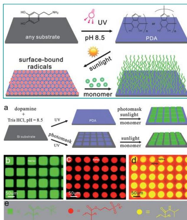
**Fig. 8** (a) Outlined procedures for preparing patterned polymers. (b) Fluorescence image of methyl orange-stained PMETAC, (c) Rhodamine 6G-stained PSPMA, (d) binary pattern of acridine-stained PSPMA/PNIPAm, and the corresponding chemical structures (e). The bright green area is PMETAC, the red area is PSPMA, the yellow area is PNIPAm. (reprinted with permission from Ref.<sup>139</sup>).
