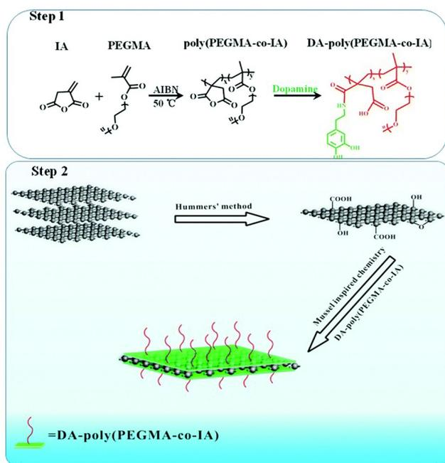
**Fig. 7** Schematic illustration of the preparation of DA-poly(PEGMA-co-IA) modified GO via mussel inspired chemistry. Step 1 shows the synthesis of poly(PEGMA-co-IA) by free radical living polymerization, which was subsequently reacted with DA to get DA-poly(PEGMA-co-IA). Step 2 illustrates the attachment of DA-poly(PEGMA-co-IA) onto GO via mussel inspired chemistry. (reprinted with permission from Ref.<sup>133</sup>).
