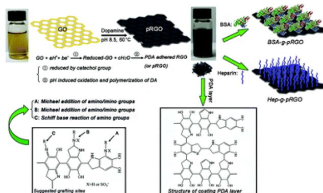
**Fig. 18** Approach for constructing the aqueous stable and biocompatible RGO by a biomimetic method, and the possible PDA chemical structure as well as the suggested reaction mechanism. Note: the PDA coating layer could immobilize the biopolymer which contained thiols, imino, and amines groups, such as heparin or protein. (reprinted with permission from Ref. <sup>84</sup>)
