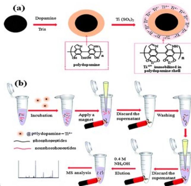
**Fig. 11** (a) Synthetic route to  $\text{Fe}_3\text{O}_4@PD\text{-Ti}^{4+}$  microspheres; (b) workflow of phosphopeptides enrichment from a biological sample using  $\text{Fe}_3\text{O}_4@PD\text{-Ti}^{4+}$  microspheres. (reprinted with permission from Ref. <sup>151</sup>).
