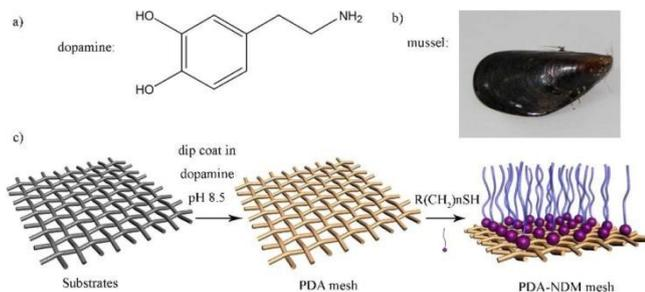
**Fig. 3** a) Chemical structure of dopamine; b) photograph of a mussel; c) schematic description of the preparation of polydopamine coated stainless steel mesh film and N-dodecyl mercaptan modified surface through Michael addition reaction. (reprinted with permission from Ref.<sup>88</sup>).
