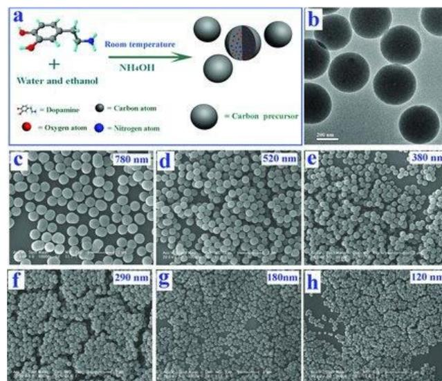
**Fig. 2** a) Schematic illustration of the synthesis of PDA SMSs. b) Typical TEM image of PDA SMSs with an average diameter of 380 nm. c–h) SEM images of PDA SMSs with different diameter prepared at different ratios of ammonia and dopamine. (reprinted with permission from Ref. <sup>46</sup>).
