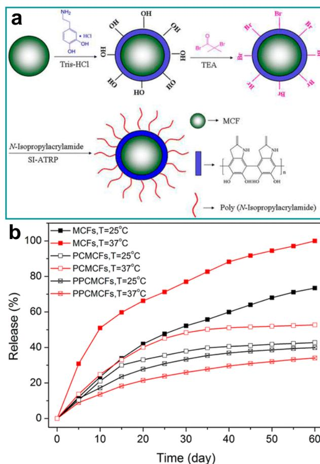
**Fig. 4** (a) Schematic illustration of the ATRP Grafted with PNIPAm from Pdp-Coated Fertilizers. (b) Stimuli-responsive release behavior of Cu from fertilizers at different temperatures. (reprinted with permission from Ref.<sup>106</sup>).
