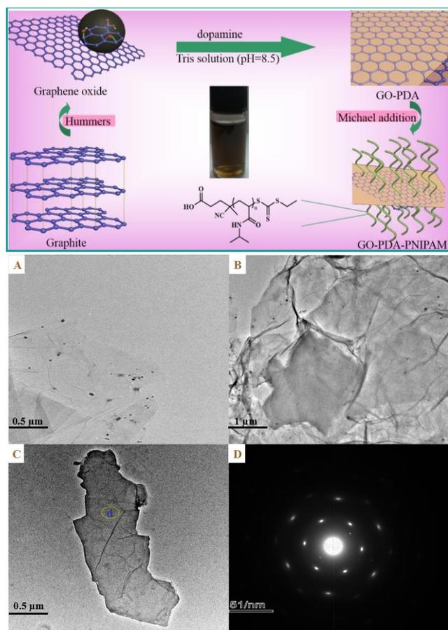
**Fig. 6** Schematic representation for the preparation of GO-PDA-PNIPAM. Step 1: graphite was first oxidized and exfoliated into a single layer of slices through a modified Hummers' method. Step 2: GO was coated with PDA in Tris solution through mussel adhesion. Step 3: the intermediate, GO-PDA, was grafted with poly(N-isopropylacrylamide) (PNIPAM) through a Michael addition reaction. (A) A TEM image of GO
