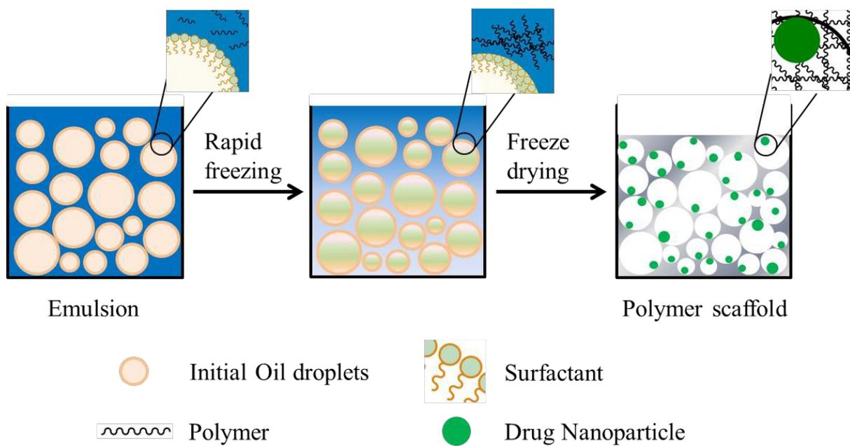
**Fig. 5** Schematic representation of the emulsion freeze drying process.
