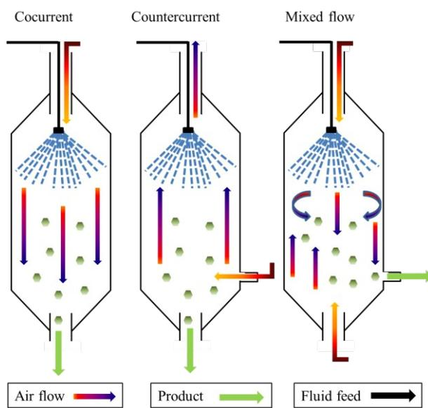
**Fig. 4** Schematic representation of spray drying apparatus with different currents.
