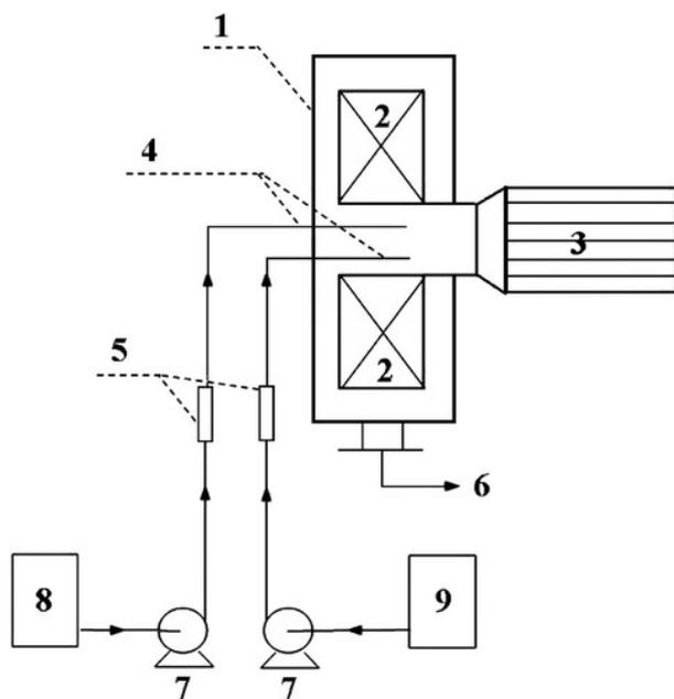
**Fig. 3** Schematic representation of high-gravity process. 1-rotating packed bed; 2-packing; 3-motor; 4-liquid distributor; 5-flow meters; 6-outlet; 7-pump; 8,9-liquid storage tank. Adapted with permission from ref. 74. © 2012 Informa Healthcare USA.
