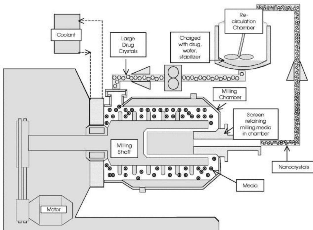
**Fig. 2** Schematic representation of the media milling process. Batch or continuous mode is possible.
