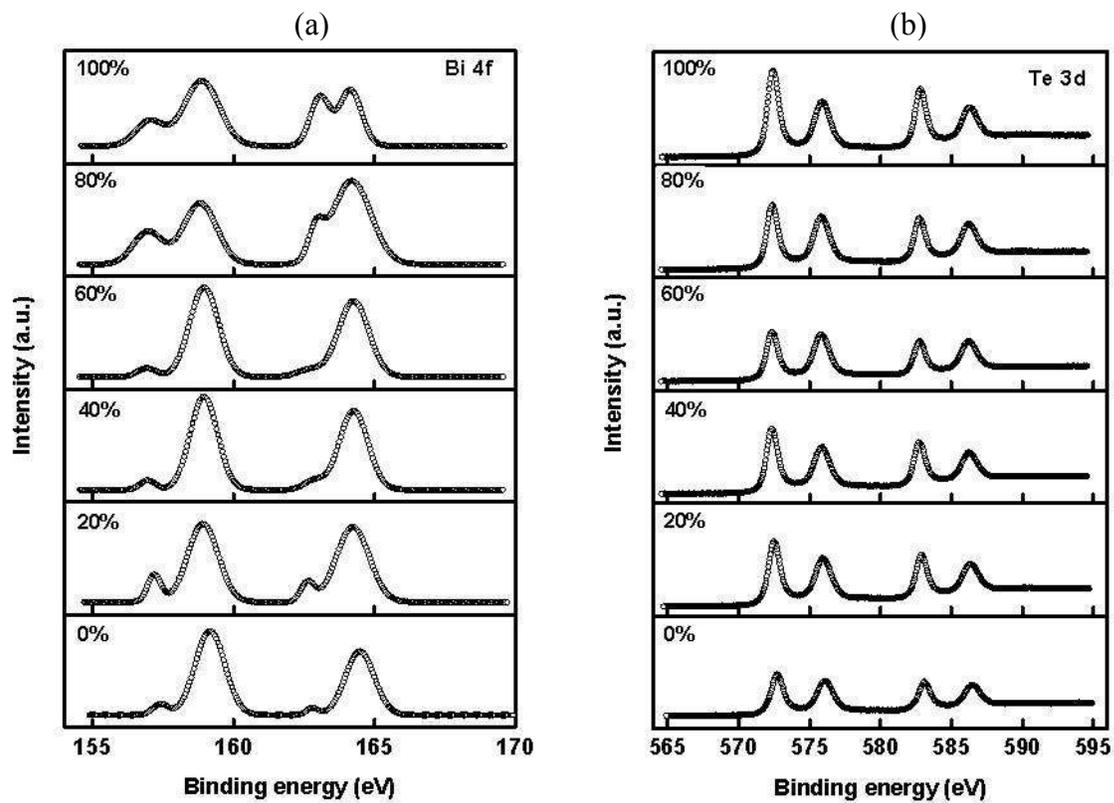
**Fig. 4** XPS spectra of Te-Bi<sub>2</sub>Te<sub>3</sub>/PEDOT:PSS hybrid films treated with various concentrations of H<sub>2</sub>SO<sub>4</sub>: (a) Bi 4f and (b) Te 3d.
