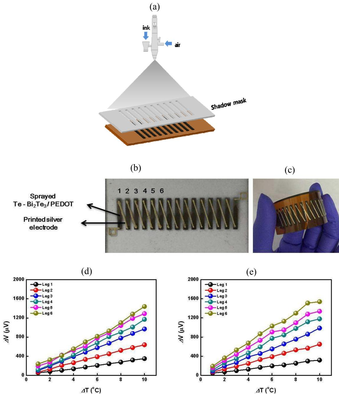
**Fig. 5** (a) Schematic drawing of the spray-printing process, (b) image of the planar thermoelectric generator consisting of 15 legs arranged on the glass substrate, (c) image of the flexible thermoelectric generator, and (d, e) open circuit thermoelectric voltage ( $V_{oc}$ ) vs. temperature difference ( $\Delta T$ ) according to the number of TE legs of rigid and flexible TE generators.
