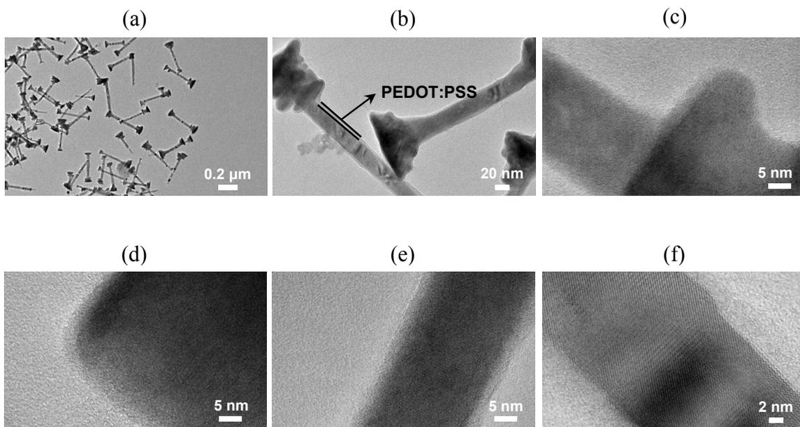
**Figure 1.** TEM images of Te–Bi<sub>2</sub>Te<sub>3</sub>/PEDOT:PSS hybrids: (a, b) nano-barbell structures of Te–Bi<sub>2</sub>Te<sub>3</sub> nanowire heterostructures coated with PEDOT:PSS, (c) the junction between the nanobar (Te) and plate (Bi<sub>2</sub>Te<sub>3</sub>) part, (d) high magnification of the plate part, (e) high magnification of the nanobar part, and (f) crystalline phase in the hybrid.
