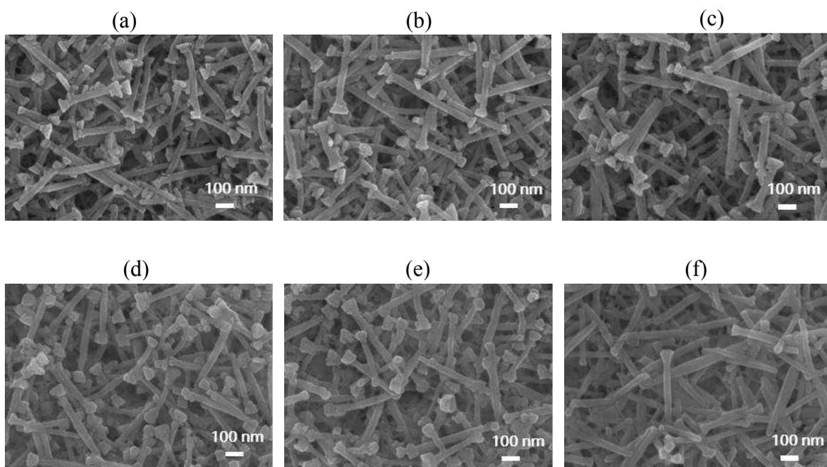
**Fig. 3** Surface SEM images of Te-Bi<sub>2</sub>Te<sub>3</sub>/PEDOT:PSS hybrid films treated with various concentrations of H<sub>2</sub>SO<sub>4</sub>: (a) 0, (b) 20, (c) 40, (d) 60, (e) 80, and (f) 100 vol%, respectively.
