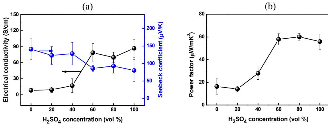
**Figure 2.** Thermoelectric properties of Te-Bi<sub>2</sub>Te<sub>3</sub>-PEDOT:PSS hybrid films treated with various concentrations of H<sub>2</sub>SO<sub>4</sub>: (a) electrical conductivity (black circle) and Seebeck coefficient (blue circle) and (b) power factor.
