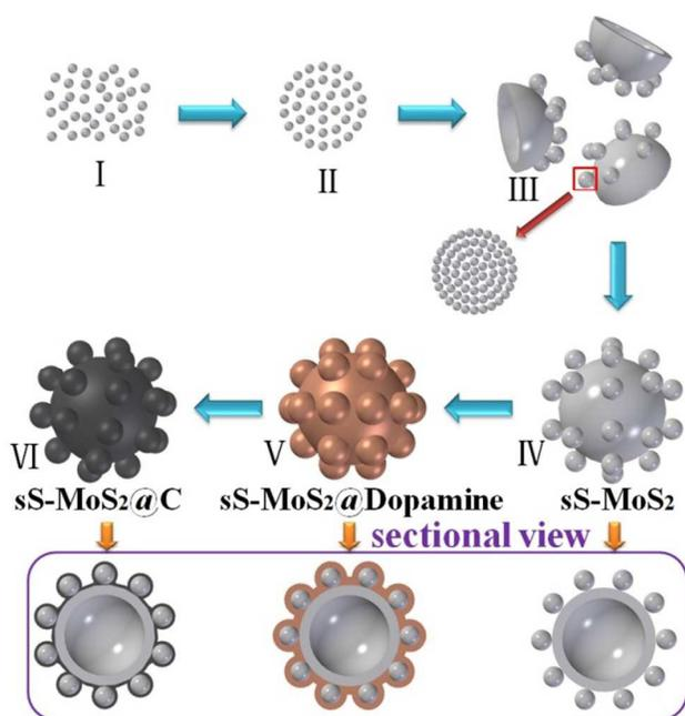
**Scheme 1.** Scheme for the fabrication of sS-MoS<sub>2</sub>@C.
