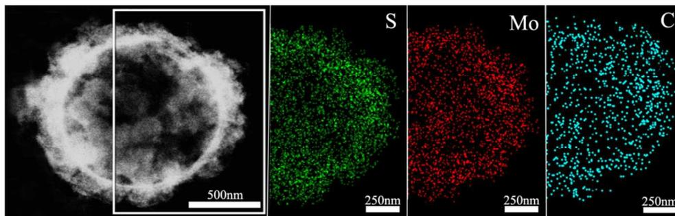
**Figure 4.** Scanning transmission electron microscopy (STEM) image of sS-MoS<sub>2</sub>@C microstructure, and the EDX mapping images of S, Mo and C elements.
