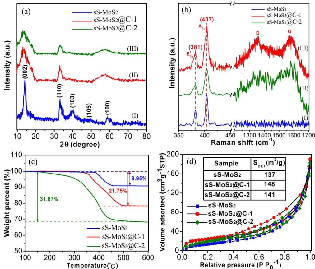
**Figure 3.** (a) XRD patterns and (b) Raman spectra of bare sS-MoS<sub>2</sub>, sS-MoS<sub>2</sub>@C-1 and sS-MoS<sub>2</sub>@C-2 composites. (c) TG curves of sS-MoS<sub>2</sub>, sS-MoS<sub>2</sub>@C-1 and sS-MoS<sub>2</sub>@C-2 under air atmosphere. (d) N<sub>2</sub> adsorption–desorption isotherms of sS-MoS<sub>2</sub>, sS-MoS<sub>2</sub>@C-1 and sS-MoS<sub>2</sub>@C-2.
