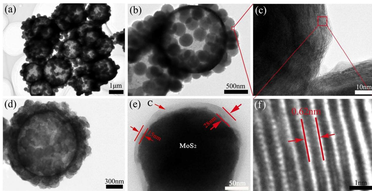
**Figure 2.** TEM images of bare sS-MoS<sub>2</sub> and sS-MoS<sub>2</sub>@C. (a) Low magnification TEM image of sS-MoS<sub>2</sub>. (b) Medium magnification TEM image sS-MoS<sub>2</sub>. (c) High-resolution TEM image of onion-like solid nanosphere. (d) Medium magnification TEM image of sS-MoS<sub>2</sub>@C-1. (e) High magnification TEM image of sS-MoS<sub>2</sub>@C-1. (f) High-resolution TEM image of sS-MoS<sub>2</sub>.
