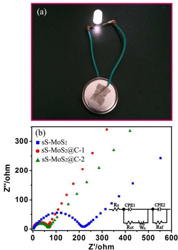
**Figure 7.** (a) Photograph of a LEDs powered by one coin cell based on the sS-MoS<sub>2</sub>@C-1 electrode. (b) Nyquist plots of the sS-MoS<sub>2</sub>, sS-MoS<sub>2</sub>@C-1 and sS-MoS<sub>2</sub>@C-2 electrodes in the frequency range from 200 kHz to 0.01 kHz.
