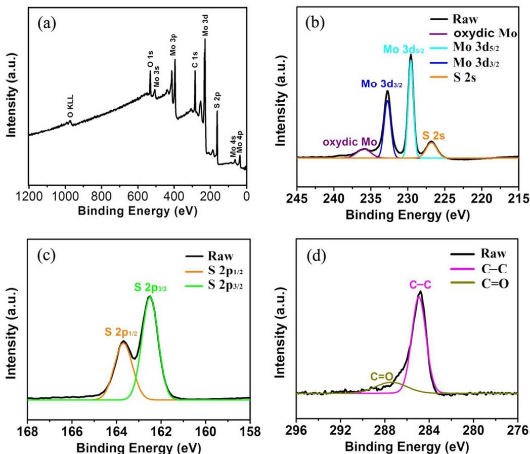
Figure 5. XPS spectra of sS-MoS<sub>2</sub>@C-1 (a) Survey spectrum. (b) Mo 3d spectrum. (c) S 2p spectrum. (d) C 1s spectrum.
