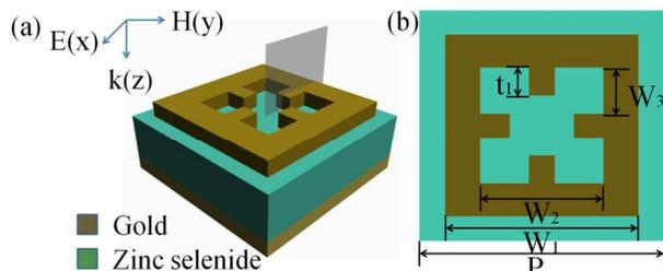
Fig. 1: Schematic of our designed absorber. (a) The units cell of the structure and (b) the detailed structural information of the unit. Here we select  $w_1=7.5\ \mu\text{m}$ ,  $w_2=4.8\ \mu\text{m}$ ,  $w_3=1.9\ \mu\text{m}$  and  $t_1=1.15\ \mu\text{m}$ .
