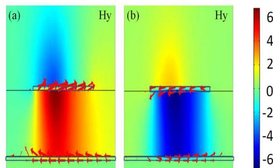
Fig. 3: The magnetic field along y-axis ( $H_y$ ) distribution and the electric displacement in the grey-plane through the middle of the patterned edge at 17.9 THz and 25.6 THz illuminated under normally TM polarized incident wave.
