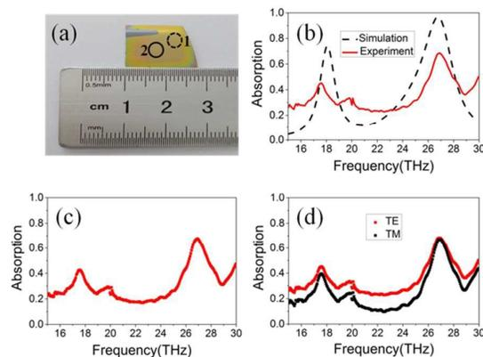
FIG.5: (a) The sample with two positions marked with 1 and 2. (b) The absorption spectra of the sample. The red solid line shows the experimental spectra of position 1 and the black dash line shows the simulation spectra by taking one unit cell of SEM image into numerical model (c) The absorption spectra of position 2. (d) The absorption spectra of position 1 under both TE and TM polarizations. The red line and the black line represent the TE and TM polarizations respectively.
