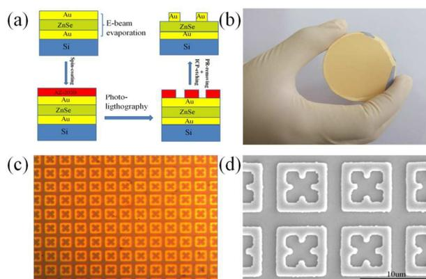
FIG.4: (a) The fabrication procedure of the metamaterial perfect absorber. (b) The picture of the whole sample. (c) The microscope image of the transfer patterns on photoresist. (d) The SEM image of the final metamaterial.
