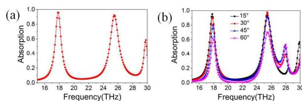
Fig. 2: (a) Absorptions spectra under normally incident TM (or TE) plane wave. (b) Absorption spectra as a function of the angle of incidence for TM (or TE) polarization plane wave.
