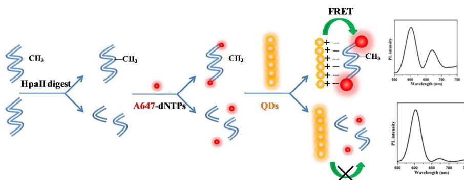
**Fig. 1** Schematic illustration of the detection of DNA methylation based on QDs-FRET.
