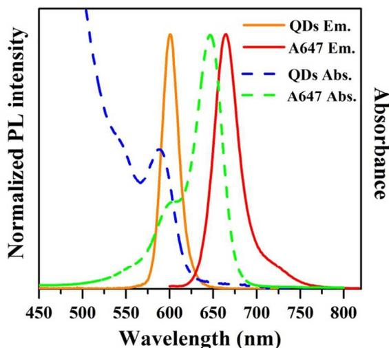
**Fig. 2** Normalized UV-vis absorption (abs) and fluorescence emission (em) spectra of A647 and amino-QDs.
