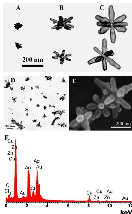
**Figure 2** Micrographs of Au/Ag HNS obtained by TEM from (A) sample A, (B) sample B, and (C) sample C. For the specific case of sample C, the general view of TEM (D), the SEM (E) images and the EDX spectrum (F) are shown.
