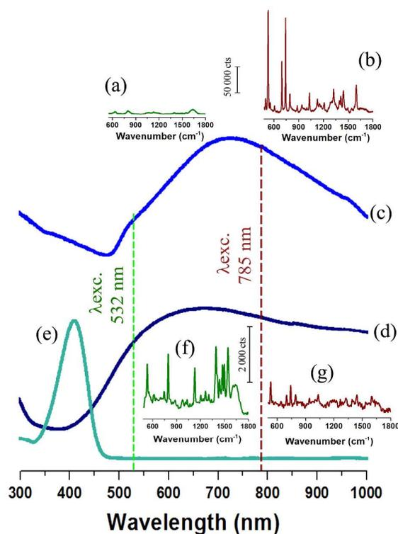
**Figure 7.** SERS spectra of ThT obtained by using different substrates and excitation lines: sample A and excitation at 532 nm (a) and 785 nm (b) and sample C and excitation at 532 nm (f) and 785 nm (g). The extinction spectra of samples A (c) and C (d) and the absorption spectrum of ThT (0.1 M) in water (e) were also shown for comparison.
