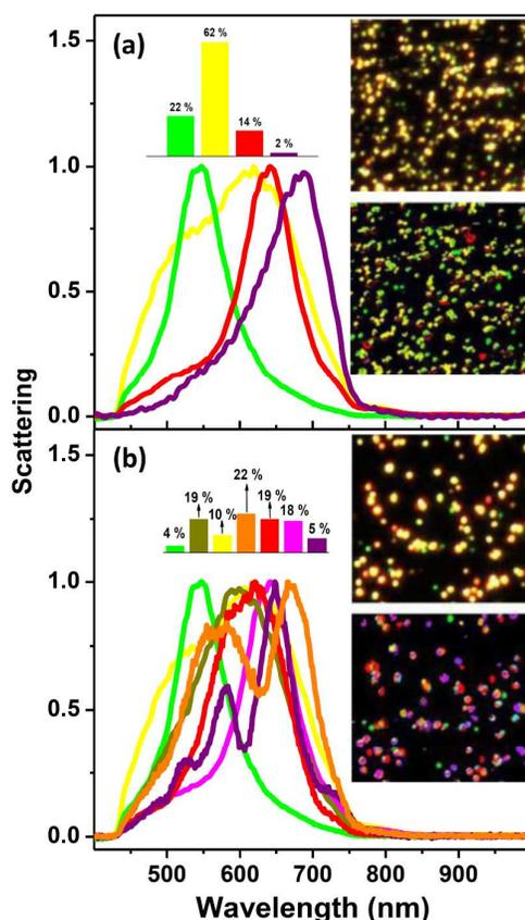
**Figure 4** The scattering spectra observed in samples: C (a) and D (b) obtained from the hyperspectral analysis. Inset: EDFM images (up) and their spectral map (down) with colored area indicating the matching with the spectral endmembers. Relative percentage abundance of the spectral profiles, revealed by the SAM analysis of the hyperspectral images, is also displayed. All the EDFM and SAM images are  $15\ \mu\text{m} \times 15\ \mu\text{m}$ .
