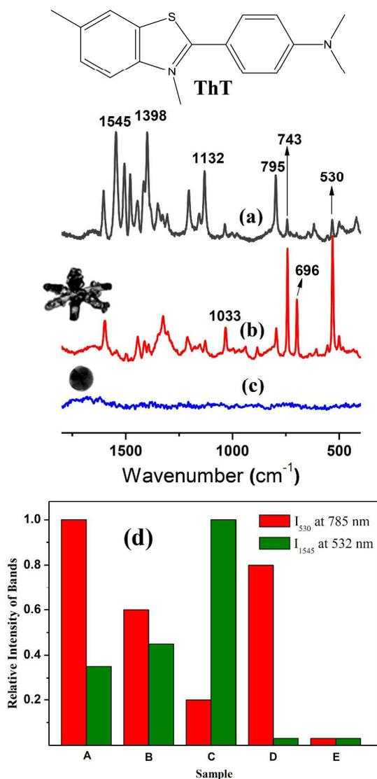
**Figure 6** Raman spectrum of ThT 10 mM (a) and the SERS spectra of ThT 1  $\mu$ M obtained on samples B (b) and E (c), at the excitation wavelength of 785 nm. (d) SERS enhancement dependence on the excitation wavelength and the colloidal suspension used: 532 nm and 785 nm. A, B, C, D and E correspond to the samples indicates in the Table 1. This enhancement dependence was normalized to the maximum value in each case.
