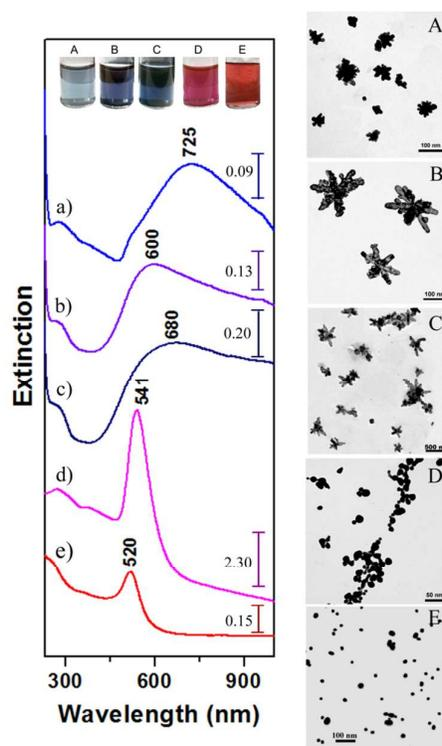
**Figure 3** Extinction spectra (left) and TEM images (right) corresponding to the samples: A (a), B (b), C (c), D (d) and E (e). *Inset*: Pictures of colloids obtained from the A, B, C, D and E samples.
