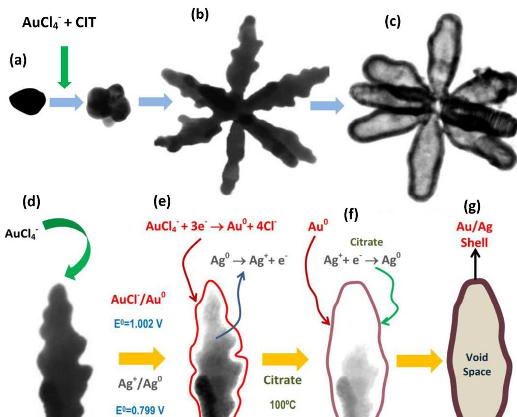
**Figure 1.** Up: (a-c) Schematic procedure suggested for the fabrication of Au/Ag hollow nanostars from Ag NS templates; Bottom: (d-g) Reaction mechanisms suggested to explain the conversion of one AgNS arm into a hollow structure, by galvanic replacement and Ag redeposition induced by residual citrate.
