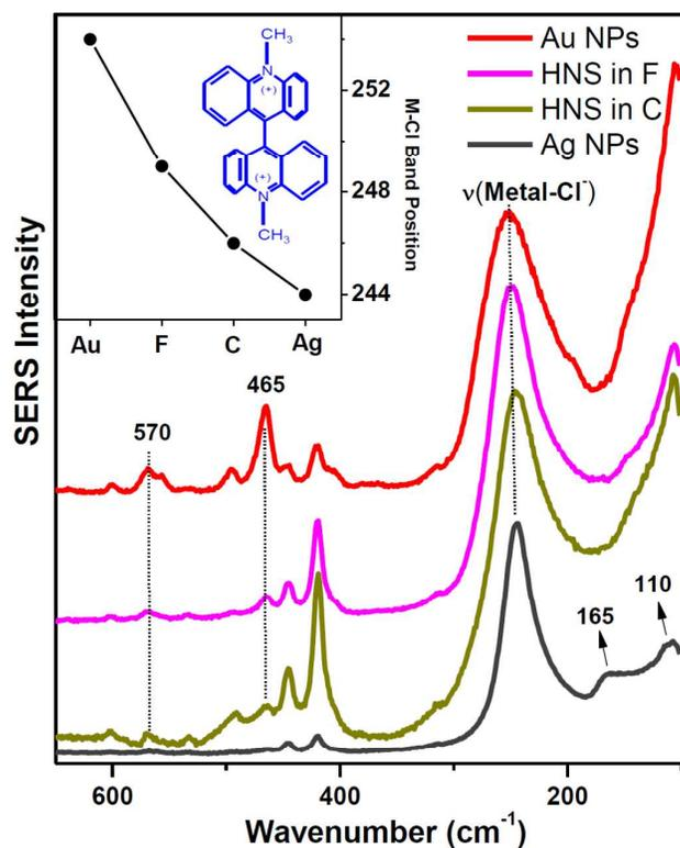
**Figure 5** Low wavenumber region of SERS spectra of lucigenin on the following metal substrates: Ag NPs, Au NPs, and HNS of samples C and F, respectively. Inset: chemical structure of lucigenin and dependence of the  $\nu(\text{Metal-Cl})$  band position in the SERS spectra obtained by using different NPs. This trend depends strongly on the Au content. These spectra were obtained by using the laser at 785 nm.
