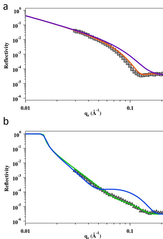
**Figure 4.** Comparison of two models of SAMs with Janus structure and uniform distribution of ligands for d-OT-MHol 1:1 coated NPs in two different subphases. a) NR profile (squares) in NRW subphase with two different models (solid lines): uniformly mixed in red and Janus in violet. b) NR profile (triangles) in CMAu subphase, showing the best two fits (solid lines) for uniformly mixed in green (□□□□84°) and Janus in blue (□□□□97°).
