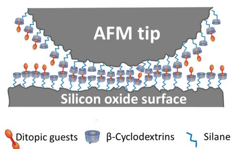
**Fig. 1** Schematic representation of a  $\beta$ -CD hosts monolayer attached to an AFM tip and silicon wafer. Hydrophobic interactions lead to inclusion of the connector molecules into the hosts and to the tip-sample interaction.
