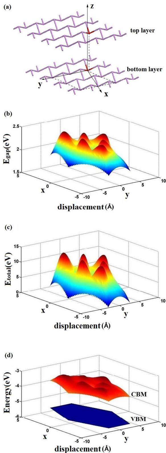
**Figure 1.** The BLBP electronic structure dependence on the lateral displacement. (a) The schematic diagram of lateral interlayer displacement in which the bottom layer standing still and top layer is moved laterally. (b-d) Three dimensional plotting of  $E_{gap}$ (b),  $E_{total}$  (c),  $E_{VBM}$  and  $E_{CBM}$  (d) when the top layer is moved laterally in x and y directions. For  $E_{VBM}$  and  $E_{CBM}$  the energy of vacuum level setting to zero.
