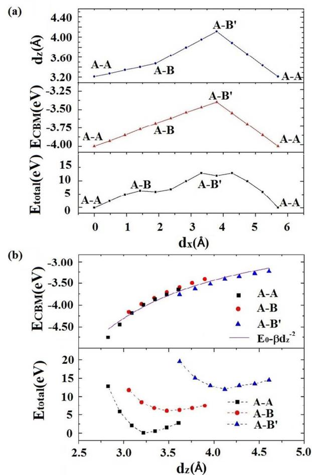
**Figure 3.** (a) The change of  $E_{total}$ ,  $E_{CBM}$  and  $d_z$  correlated with the lateral interlayer displacement  $d_x$  on the route of A-A – A-B – A-B' – A-A. (b) The change of  $E_{total}$  and  $E_{CBM}$  correlated with  $d_z$  for the vertical interlayer displacement of A-A, A-B and A-B' stacking configurations. The fitting of  $E_{CBM} = E_0 - \beta d_z^{-2}$  is also shown.
