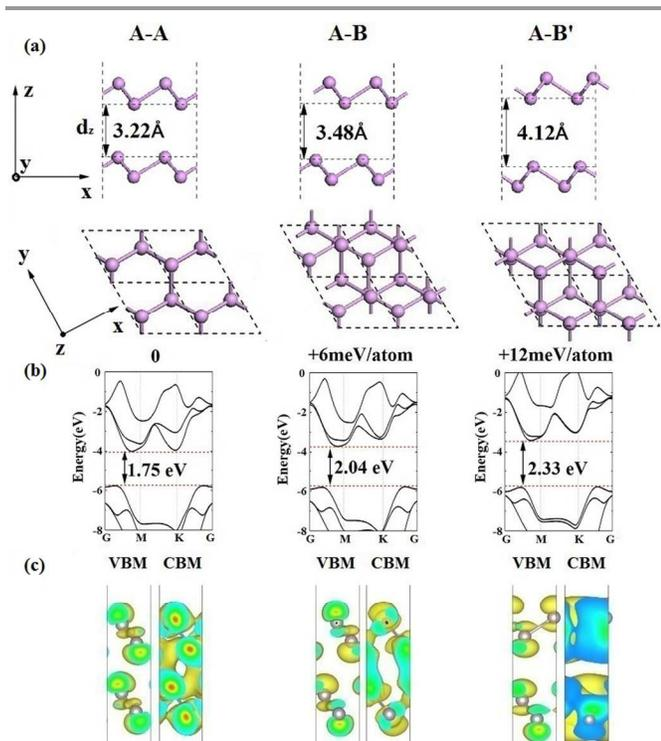
**Figure 2.** Atomic geometries structures (a), band structures (b) and orbital probability density distributions of VBM and CBM (c) of A-A, A-B and A-B' stacking BLBP. Corresponding  $E_{total}$ ,  $E_{gap}$  and  $d_z$  are also given. The  $E_{total}$  of A-A stacking is set to zero. For the orbital probability density distribution iso-surface plotting, the iso-value is 0.004 e/au<sup>3</sup>.
