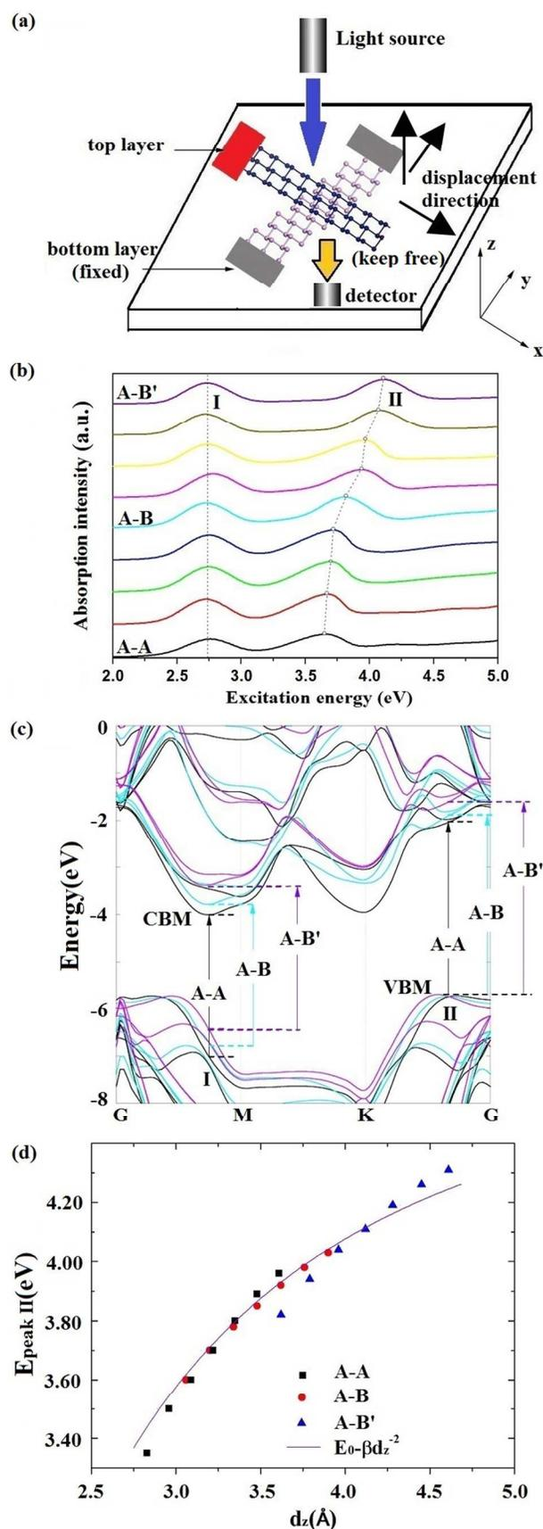
**Figure 4.** (a) The schematic design diagram of the nano-scale displacement sensor based on BLBP. (b-c) The absorption intensity (b) and band structure (c) of BLBP when the top layer is moved laterally from A-A (black line) through A-B (cyan line) to A-B' (purple line). (d) The change of  $E_{\text{peakII}}$  correlated with  $d_z$  for the vertical interlayer displacement of A-A, A-B and A-B' stacking configurations. The fitting of  $E_{\text{peakII}} = E_0 - \beta d_z^{-2}$  is also shown.
