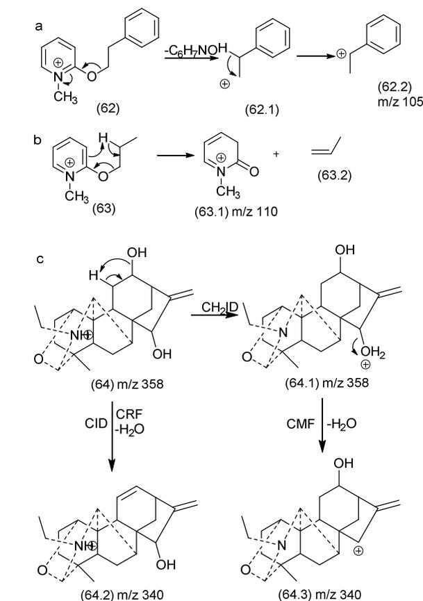
1115 Fig. 32 Retro-ene (CRF) reactions in alkyl 1-methylpyridinium ions (a and b) and competition between CRF and CMF in diterpenealkaloids (c).
