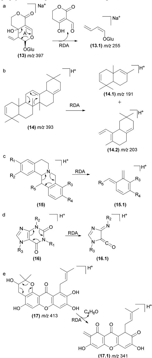
640 Fig. 10 RDA fragmentation in terpenoids limonoids (a), saponins (b), isoquinolinealkaloids (c), caffeine (d), and polyprenylatedxanthones (e).
