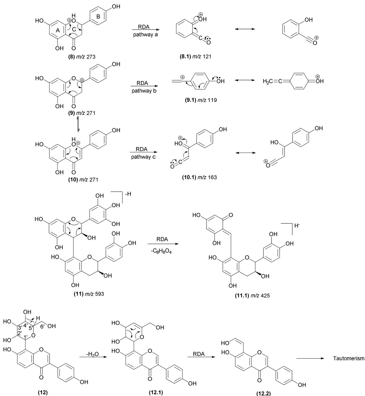
620 Fig. 9 RDA mechanisms involving the C-ring of flavonoids (**8-10**) and proanthocyanidins (**10**) and sugar units in natural products (**12**). The double bond present in the C-ring of flavones, flavonols, chalcones and isoflavones leads to an additional pathway (pathway c).
