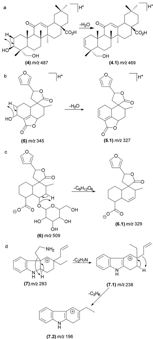
605 Fig. 8 Remote hydrogen rearrangements involved in the dehydration of saponins (a), diterpenes (b), glycosylated diterpenes and protonated plumeran alkaloids with the loss of a chain side (d).
