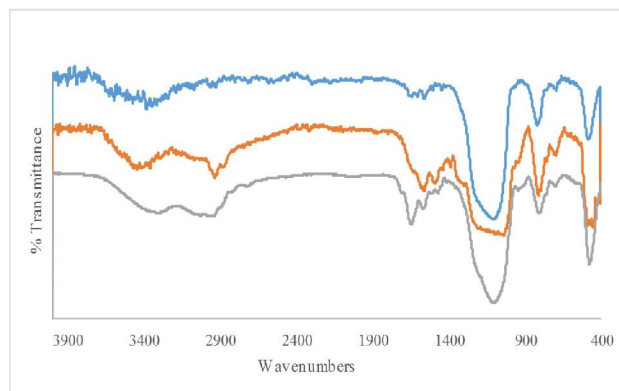
Fig. 1 (a) Infrared spectra of Fumed silica (FS), (b) silica modified with 3-(aminopropyl)trimethoxysilane (FS-APTMS) and (c) Deferasirox anchored on FS-APTMS (FS-APTMS-DFX).
