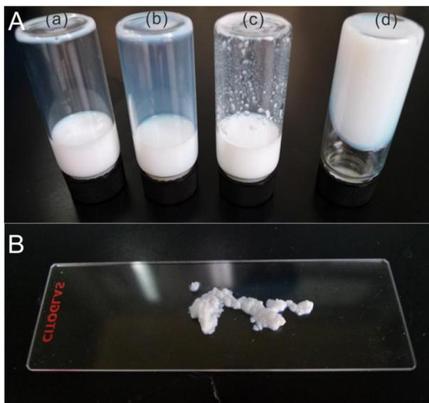
**Fig. 2** (A) Thickening process of A1, (a) A1,  $X_{20.0}Y_0Z_0$  (b) A1 added with DMEA (100% neutralization degree),  $X_{20.0}Y_{0.27}Z_0$ , (c) A1 added with 9 wt% EGBE,  $X_{20.0}Y_0Z_{1.80}$ , (d) A1 added with both DMEA (100% neutralization degree) and 9 wt% EGBE,  $X_{20.0}Y_{0.27}Z_{1.80}$ , (B) the white precipitation in the dispersion of A1 added with 9 wt% EGBE,  $X_{20.0}Y_0Z_{1.80}$ .
