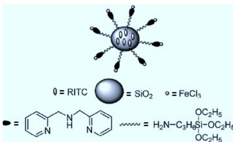
**Fig. 24:** Synthesis of RBITC-SiO<sub>2</sub>@dpa-Fe nanoparticulate systems. (Reproduced with permission from Elsevier, copyright 2015).
