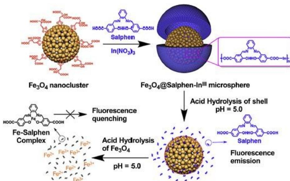
**Fig. 25:** Synthesis of Fe<sub>3</sub>O<sub>4</sub>@Salphen-In(III) CPPs and progressive degradation of salphen-In(III) CPP shell and Fe<sub>3</sub>O<sub>4</sub> nanocluster core at 5.0 pH. (Reproduced with permission from Elsevier, copyright 2015).
