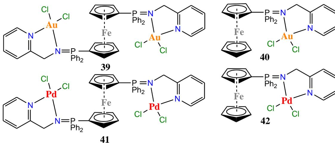
**Fig. 11:** Trimetallic (**39** and **41**) and bimetallic (**40** and **42**); gold(III) (**39** and **40**), and palladium(II) (**41** and **42**) heterometallic complexes containing iminophosphorane ligands [87].
