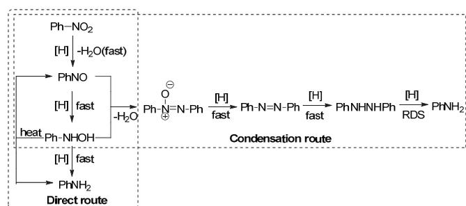
**Scheme 2.** Postulated reaction pathway for the transfer hydrogenation of nitrobenzene.
