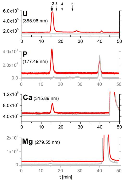
**Figure 2.** Size-exclusion LC-ICP AES of serum incubated with uranium (red) and control serum (black): a) uranium (385.96 nm); b) phosphorous (177.49 nm); c) calcium (315.89 nm), and d) Mg (279.55 nm). To correlate the approximate MW and the elution volume the standards were placed: 1) BlueDextran 2000, 2) 669 kDa, 3) 440 kDa, 4) 158 kDa and 5) 75 kDa.
