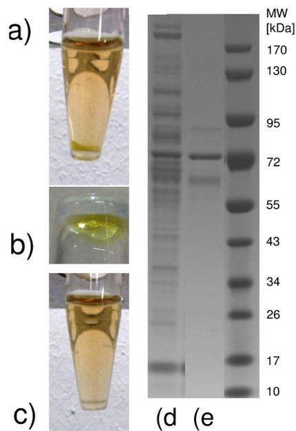
**Figure 3.** Formation of a pellet during centrifugation (12,000 rpm at 20°C) of serum incubated with: a)  $\text{UO}_2^{2+}$  species (after 180 min), b) higher-magnification view of the pellet; c) control serum; d) SDS electropherogram of the pellet (washed with 0.15 M NaCl at 4°C); e) SDS electropherogram of control serum (the serum was diluted until the intensity of three albumin bands reached that in Fig. 3d).
