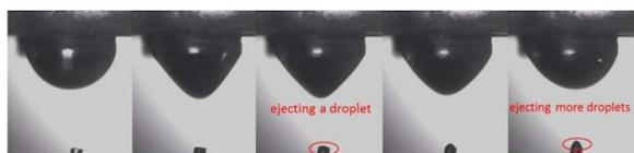
**Figure 6.** Forward EHD jet printing of a few pico-droplets on aligned optical fibre.
