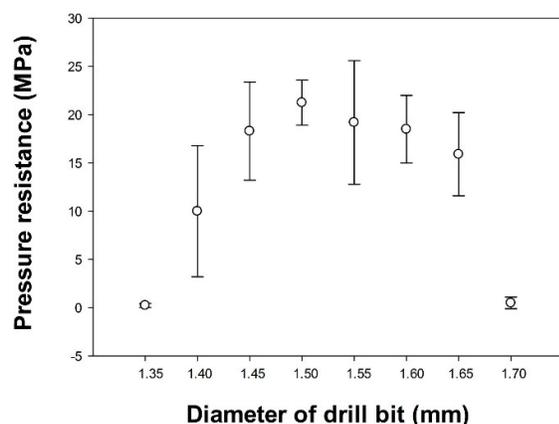
**Fig. 2.** A pressure resistance test was used to confirm what size pre-drilled hole should be used to fabricate the threaded interface at the loading reservoir. The maximum mean pressure resistance with relatively low variation ( $21.25 \pm 2.33$  MPa) was obtained using a 1.50 mm diameter drill bit to pre-drill the hole before tapping ( $n = 7$ ).
