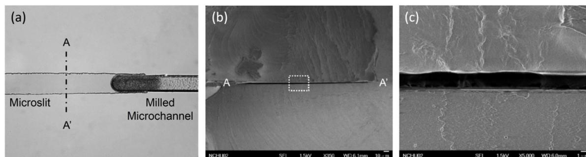
**Fig. 4.** Images of the fabricated low-aspect-ratio microfilter that were taken on a (a) optical microscope and (b), (c) SEM. A–A' cross-section was obtained using a freeze-fractured method to break the COP chip in liquid nitrogen. The SEM images show a low-aspect ratio filter, 2  $\mu\text{m}$  in height, which is formed after 30 min UV/ozone modification followed by 6 min of cyclohexane exposure.
