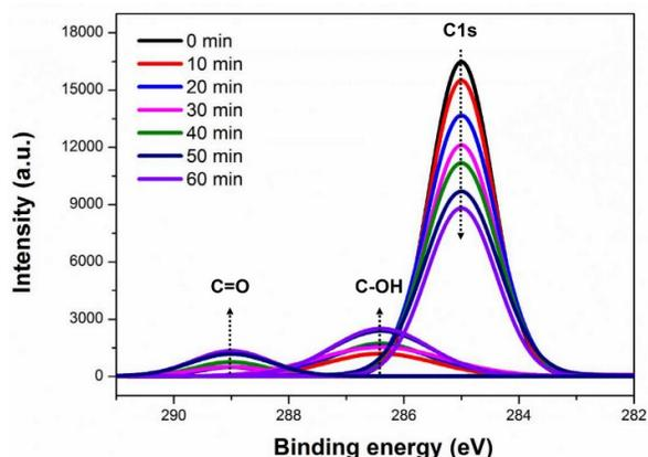
**Fig. 3.** XPS spectra of a UV/ozone oxidized COP chip surface. The C1s (main peak component C–C/C–H, 285 eV) continuously converted into C=O (289 eV) and C–OH (286.4 eV) with increasing UV/ozone exposure time.
