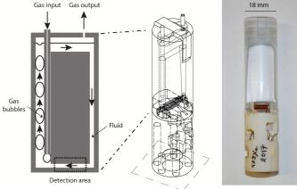
**Fig.2** The NMR cell. The principle of the bubble pump (in its top part) is depicted on the left. Middle: 3D drawing of the whole cell; right: picture of one of these cells equipped with a  $^{129}$ Xe solenoid coil.
