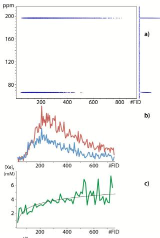
**Fig. 4** a) <sup>129</sup>Xe NMR experiment performed with a 1.3 mM solution of cryptophane-222 hexa-carboxylate and a gas flow rate of 1 mL/min. Two consecutive spectra are separated by 0.5 second. b) Areas of the signals of dissolved xenon (in red) and of xenon in cryptophane (in blue). c) Estimation of the instantaneous concentration of xenon in solution from these signal areas.
