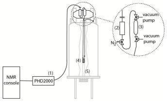
**Fig.1** Device for driven-flow of gas-loaded solutions into an NMR magnet. A syringe pump, whose console (1) is connected to the NMR console, pushes in a controlled way *via* a buffer gas (2) the gas of interest contained in a reservoir (3) to the NMR cell containing the solution (4). This cell is connected to the NMR probe head (5).
