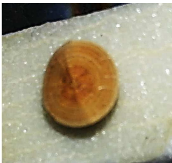
Fig. 1. Gallstone sample was placed on a gluey substance to avoid the displacement of GS test samples under the high power laser fluence.
