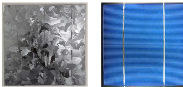
Fig. 10 Image of an reclaimed wafer obtained by the recovery processes (left) and remanufactured solar cell with reclaimed wafer (right).
