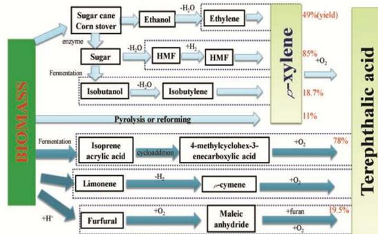
Scheme 5 Different routes for terephthalic acid synthesis from biomass
