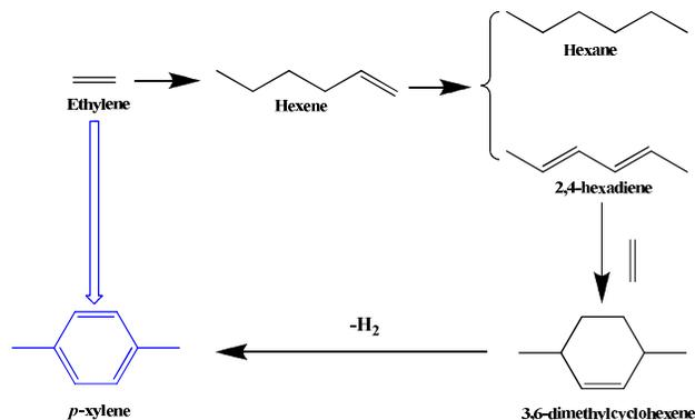
Scheme 6 Synthesis of *p*-xylene from ethylene (modified from ref.<sup>160</sup>)
