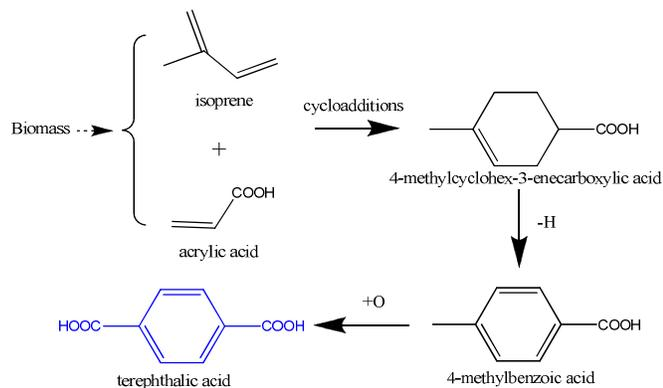
Scheme 9 Synthesis of PTA from isoprene and acrylic acid (modified from ref. <sup>246</sup>)
