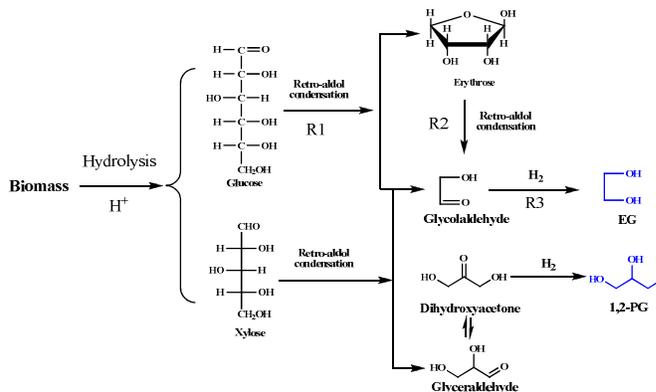
Scheme 4 The reaction pathway for conversion of cellulose and hemicellulose to EG. (modified from ref. <sup>131</sup>)
