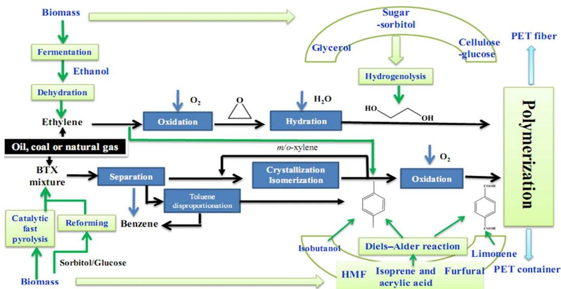
Scheme 1 Drop-in replacement of fossil based PET monomers from biomass
