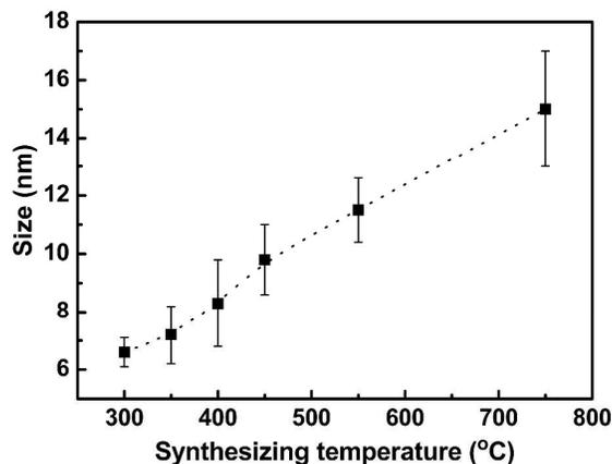
Figure 3. The average particle diameters of the particles prepared at different temperatures
