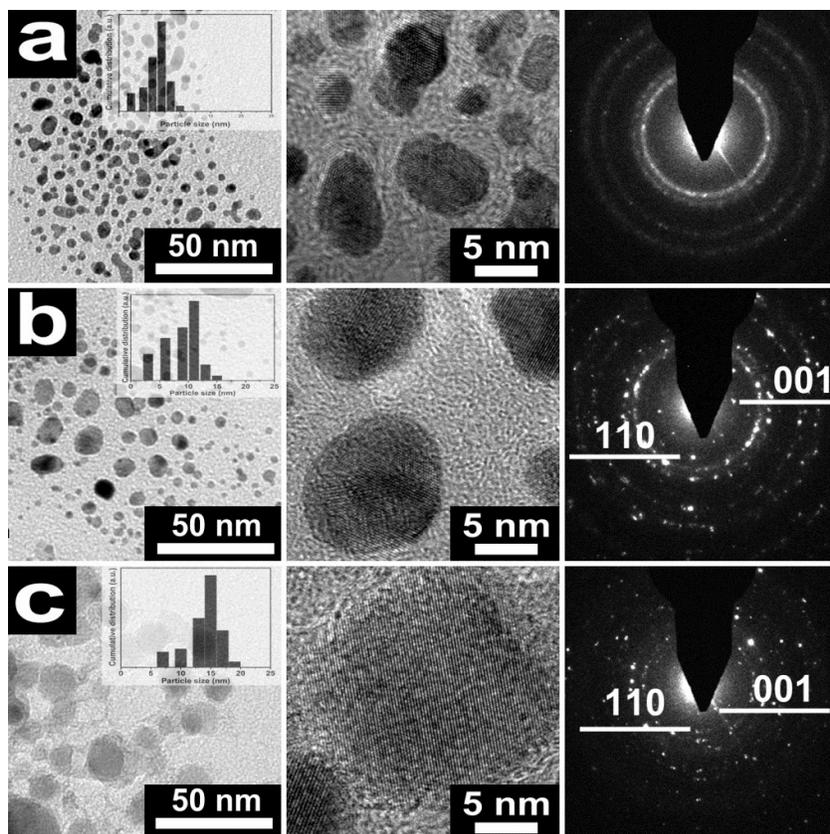
Figure 4. TEM, HRTEM and SAD images of the FePt NPs obtained at 350 °C (a), 550 °C (b), 750 °C (c). The insets show the size distribution of the particles. In each case, at least 300 particles were counted to determine the size and size dispersion.
