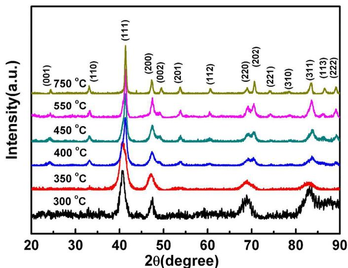
Figure 2. X-Ray diffraction patterns of the FePt nanoparticles prepared at 300 °C, 350 °C, 400 °C, 450 °C, 550 °C and 750 °C after removing the sodium chloride.
