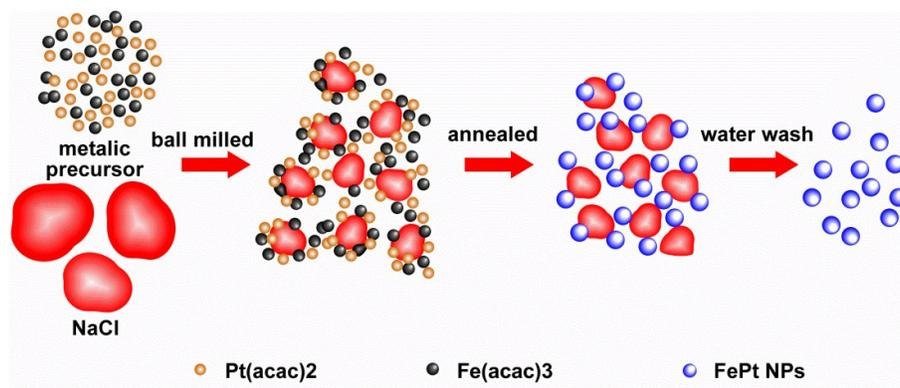
Figure 1. Schematic representation of the synthesizing of L1<sub>0</sub>-FePt nanoparticles.
