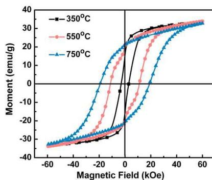
Figure 6. Room temperature hysteresis loops of the FePt NPs prepared at temperatures of 350 °C, 550 °C and 750 °C, respectively
