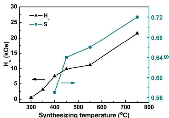
Figure 7. Temperature dependence of coercivity  $H_c$  and chemical ordering degree  $S$  of the prepared FePt nanoparticles
