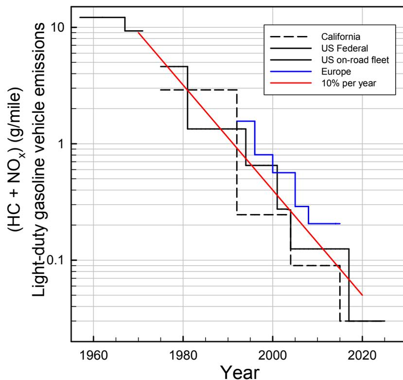
**Figure 6:** Emission standards from gasoline light-duty vehicles. Data taken from Feagraus et al. [40] and TransportPolicy.net website (<http://transportpolicy.net>). See text for details.
