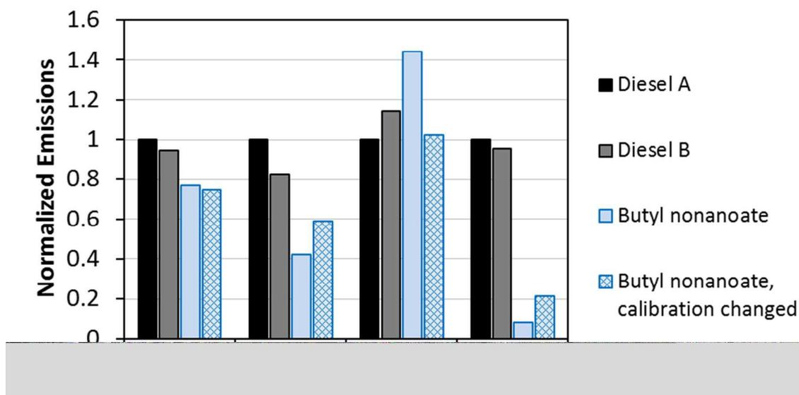
Figure 3. Engine-out emissions of THC, CO, NO<sub>x</sub>, and PM for the US06 driving cycle for the three fuels for the three fuels after engine calibration with diesel A. The right-most bar represents emissions for butyl nonanoate after adjusting the calibration to account for heating value differences as described in the text. All emissions (mg/mile) are normalized to the emissions for diesel A with the original calibration.
