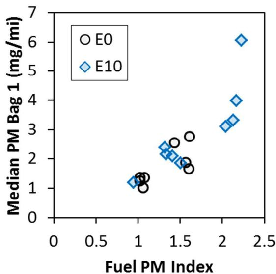
Figure 5: PM emissions from E10-capable vehicles on LA92 cycle (bag 1) when fueled with either E0 (black circles) or E10 (blue diamonds) as functions of fuel T50.
