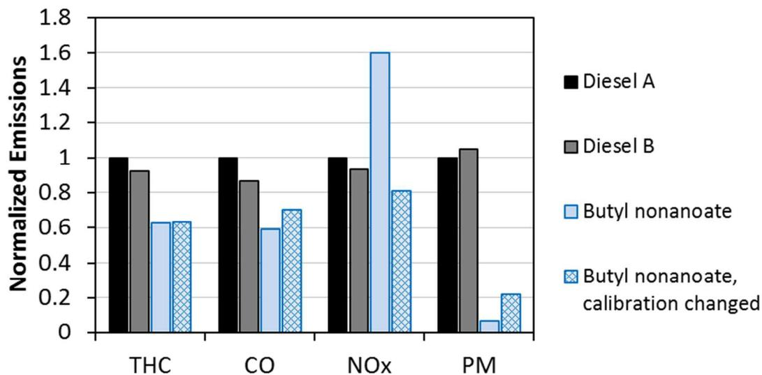
Figure 2. Engine-out emissions of THC, CO, NO<sub>x</sub>, and PM for the Highway Fuel Economy Test (HWFET) for the three fuels for the three fuels after engine calibration with diesel A. The right-most bar represents emissions for butyl nonanoate after adjusting the calibration to account for heating value differences as described in the text. All emissions (mg/mile) are normalized to the emissions for diesel A with the original calibration.
