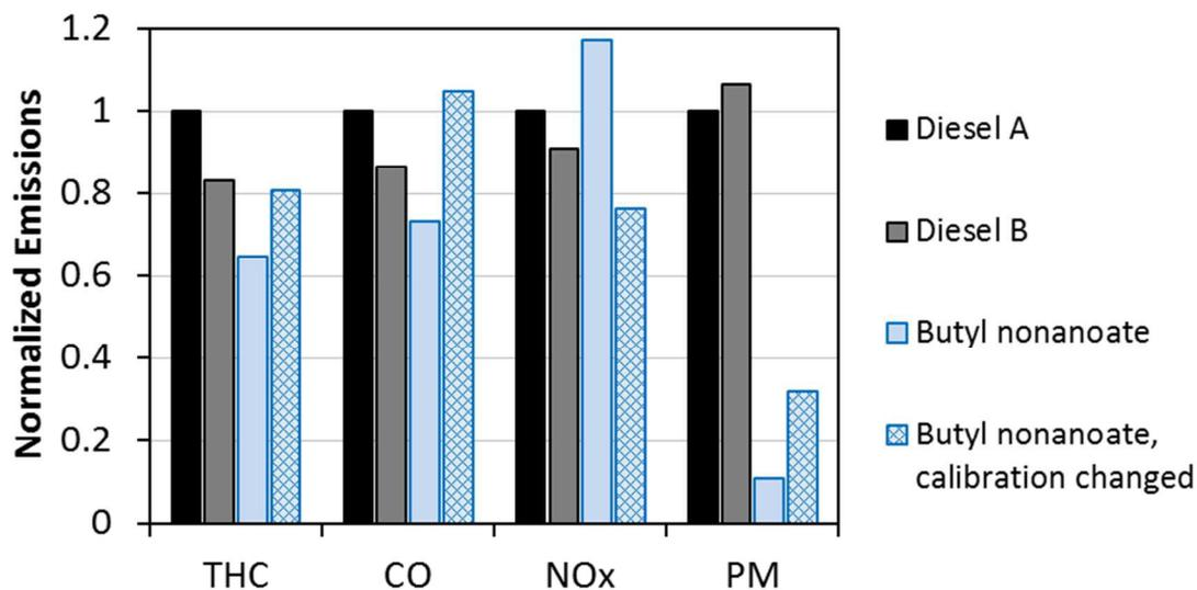
Figure 1. Engine-out emissions of THC, CO, NO<sub>x</sub>, and PM for the Federal Test Procedure (FTP-75 bag-weighted average) for the three fuels after engine calibration with diesel A. The right-most bar represents emissions for butyl nonanoate after adjusting the calibration to account for heating value differences as described in the text. All emissions (mg/mile) are normalized to the emissions for diesel A with the original calibration.
