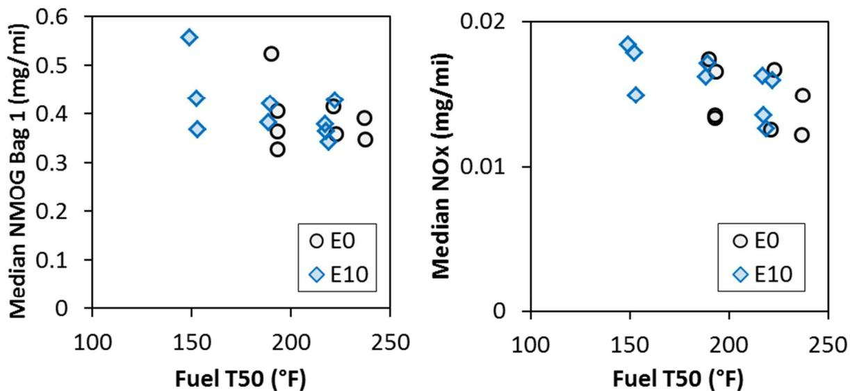
Figure 4: NMOG and NOx emissions from E10-capable vehicles on LA92 cycle when fueled with either E0 (black circles) or E10 (blue diamonds) as functions of fuel T50.
