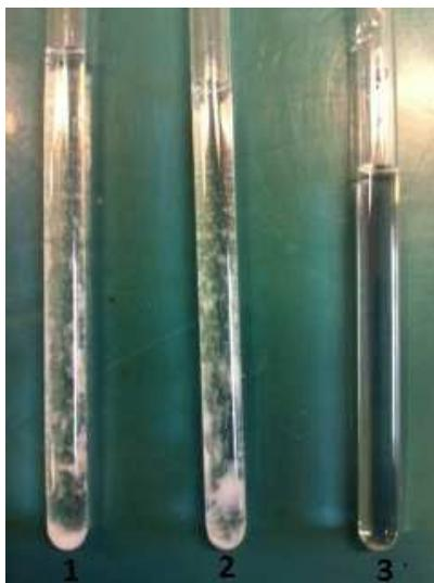
Figure 8 - The experimental solutions after 48 hours of  $^{29}\text{Si}$  NMR experiment: tubes "1" and "2" show the samples diluted with sodium chloride (at the 1.14 and 0.68 Si/M molar ratio respectively), tube "3" is the sample diluted with  $\text{H}_2\text{O}$  at the 0.68 Si/M.
