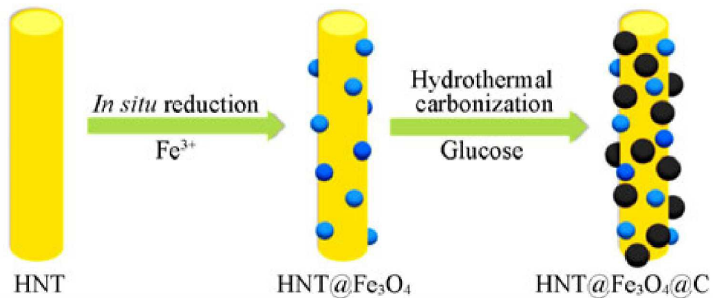
Fig. 6 Schematic showing of synthesis of HNTs/Fe 3 O 4 /carbon nanocomposite 68
