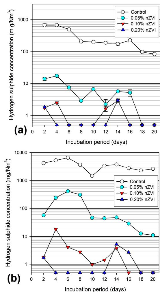
Fig. 4. Effect of NZVI doping on hydrogen sulphide concentration in biogas (a: without sulphate addition, b: with the addition of 1000 mg/L sodium sulphate).
