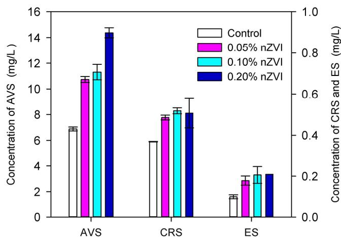
Fig. 9 The effects of NZVI-dosing on the distribution of reduced inorganic sulphur (RIS) species in sludge after anaerobic digestion.
