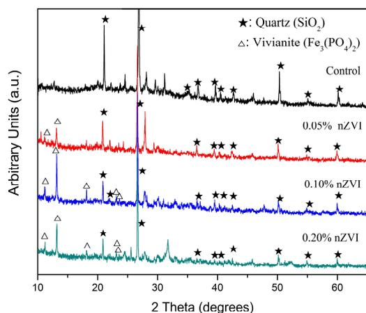
Fig. 7. XRD spectra of the crystalline phases in sludge after anaerobic digestion.
