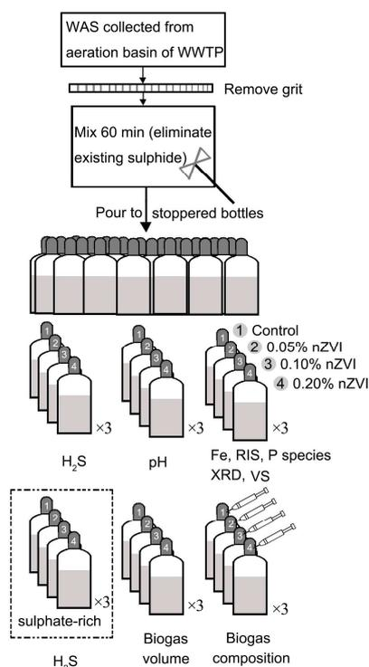
Fig. 2. Schematic description of the experimental laboratory procedure
