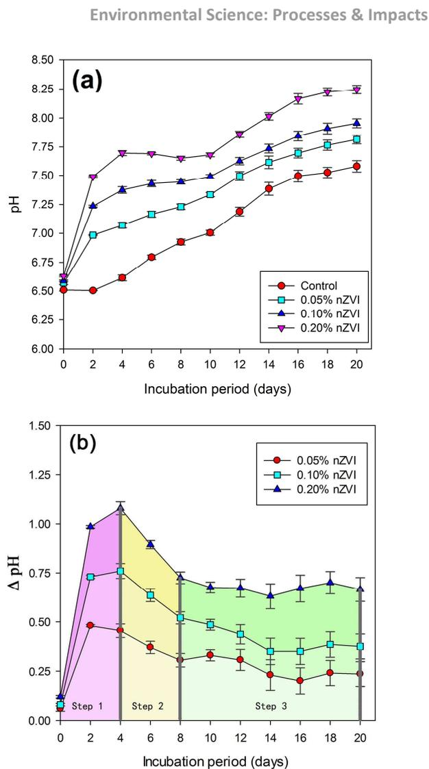
Fig. 3. The pH trends of sludge in the presence of NZVI during anaerobic digestion.
