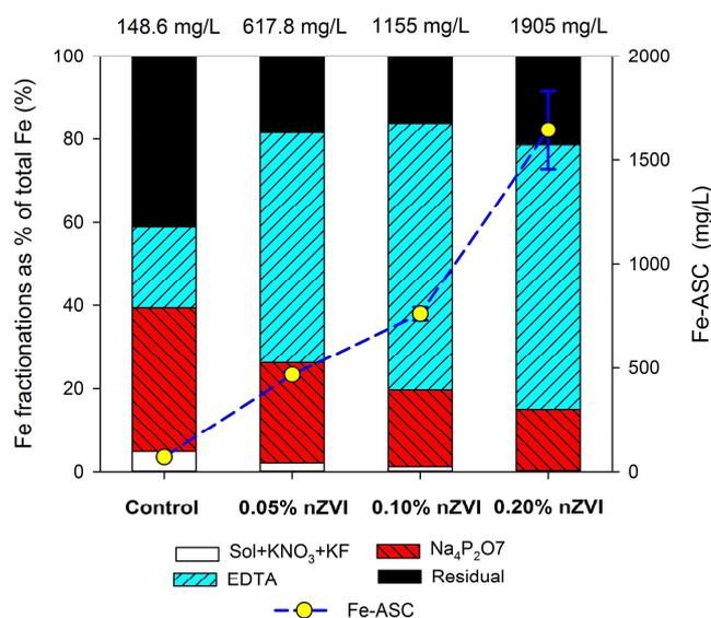
Fig. 8 The effects of NZVI-dosing on the distribution of iron in sludge after anaerobic digestion. Interpretation of iron species<sup>38</sup>,  $\text{Na}_4\text{P}_2\text{O}_7$ -Fe: Organically-bound Fe; EDTA-Fe: iron hydroxides and Fe-hydroxy-phosphates; and Residual Fe: tailings from Fe-P, Fe phosphate and FeS
