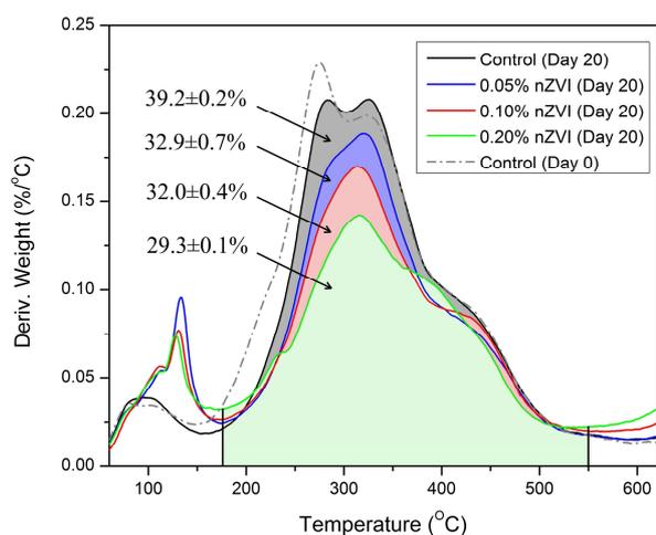
Fig. 6. TG-DSC curves of sludge at 20 d
