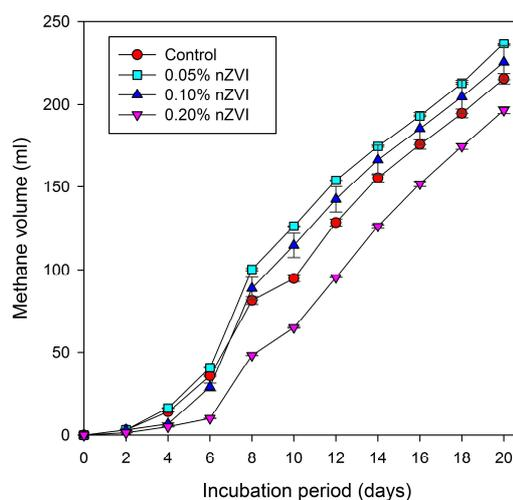
Fig. 5. The final cumulative volumes of methane produced during 20-d anaerobic digestion.
