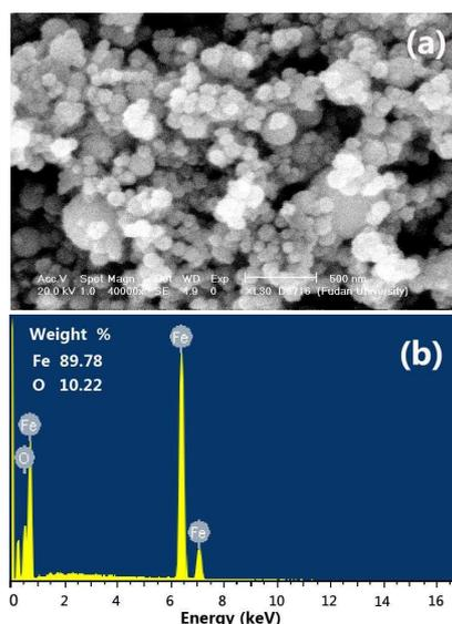
Fig. 1 SEM-EDS spectra of NZVI (40000 $\times$ )
