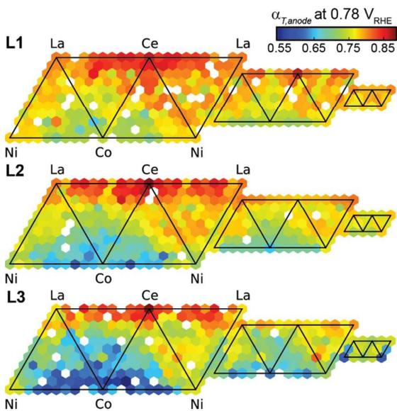
Fig. 9. Composition maps of the transmission efficiency ( $\alpha_{T,anode}$ ) of AM 1.5 irradiance through each photoanode. The optical transmission spectrum for each sample was acquired *in situ* at 0.78 V vs RHE during the anodic sweep of the chopped illumination CV.
