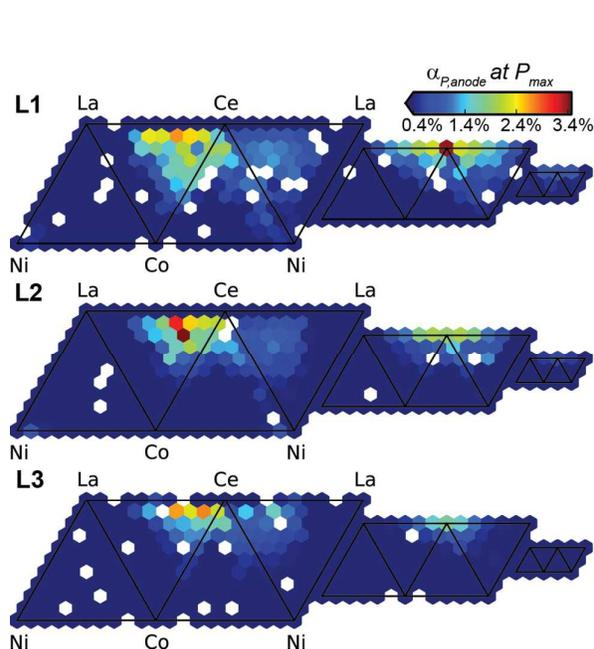
Fig. 10. Power conversion efficiency ( $\alpha_{P,anode}$ ) for each photoanode at its maximum power point. The conversion efficiency is calculated as the ratio of the maximum electrochemical power generation ( $P_{max}$ ) to the consumed optical power (reflected or absorbed irradiation,  $P_{consumed}$ ). For bare BiVO<sub>4</sub>, this efficiency is below the colour scale at 0.16%.
