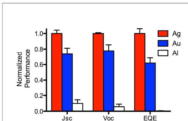
**Fig. 3** Performance of Ag, Au, and Al as evaporated cathodes in PAni-PSI/TiO<sub>2</sub> solid-state devices. For clarity, each metric was normalized to the highest performing electrode material. Error bars represent the standard error of a minimum of 4 replicates.
