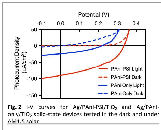
**Fig. 2** I-V curves for Ag/PAni-PSI/ $\text{TiO}_2$  and Ag/PAni-only/ $\text{TiO}_2$  solid-state devices tested in the dark and under AM1.5 solar
