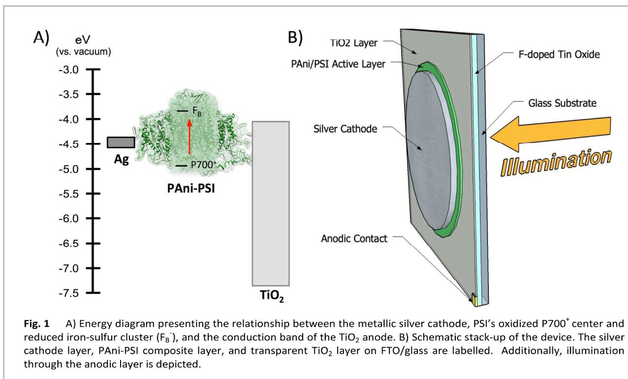
**Fig. 1** A) Energy diagram presenting the relationship between the metallic silver cathode, PSI's oxidized P700<sup>+</sup> center and reduced iron-sulfur cluster (F<sub>B</sub><sup>-</sup>), and the conduction band of the TiO<sub>2</sub> anode. B) Schematic stack-up of the device. The silver cathode layer, PANi-PSI composite layer, and transparent TiO<sub>2</sub> layer on FTO/glass are labelled. Additionally, illumination through the anodic layer is depicted.
