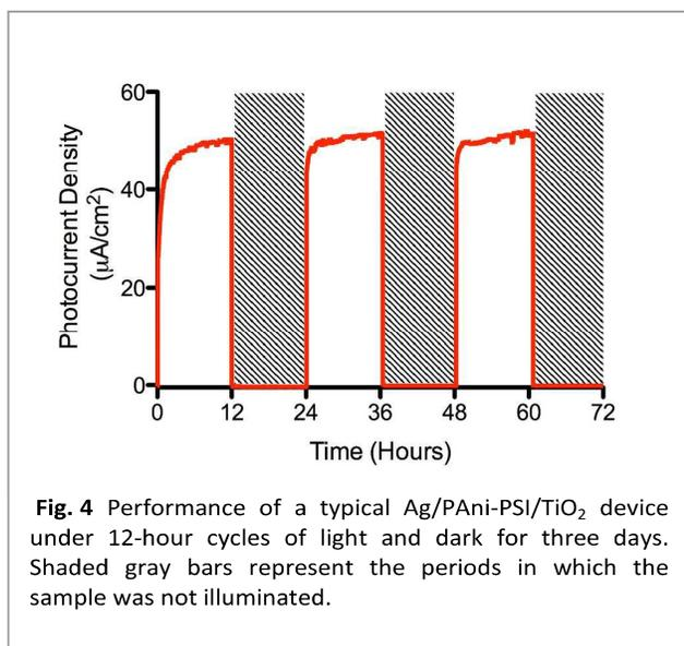
**Fig. 4** Performance of a typical Ag/PAni-PSI/TiO<sub>2</sub> device under 12-hour cycles of light and dark for three days. Shaded gray bars represent the periods in which the sample was not illuminated.
