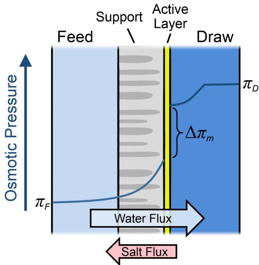
**Fig. 3** (A) Schematic diagram of the membrane channel cross section. The directions of water flux and reverse salt flux are indicated. The approximate osmotic pressure profiles along the thickness of the channel are also shown where  $\pi_F$  is the bulk feed osmotic pressure,  $\pi_D$  is the bulk draw osmotic pressure, and  $\Delta\pi_m$  is the osmotic pressure difference across the membrane active layer.
