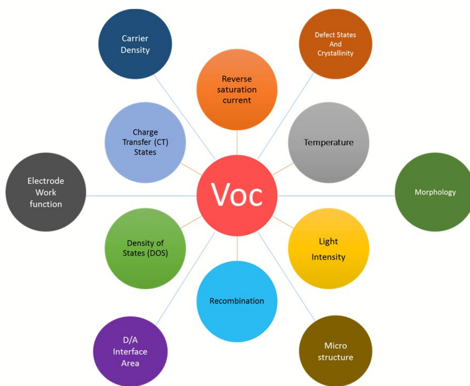
Schematic 2: Factors influencing the open circuit voltage ( V_{OC} ) in organic solar cells. Each parameter influences the V_{OC} either directly or indirectly via interrelated dependencies among them.
