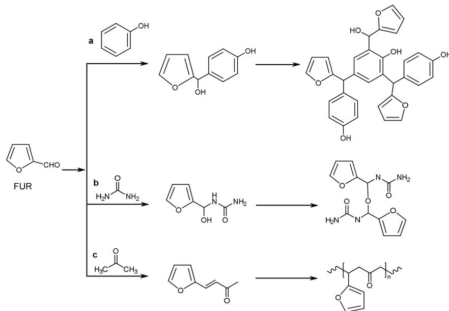
**Figure 36.** Co-polymerization of furfural (FUR) with selected monomers.
