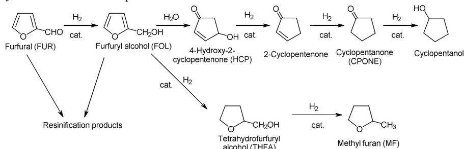
**Figure 20.** Reaction network involved in the hydrogenation of furfural (FUR) to cyclopentanone (CPONE).
