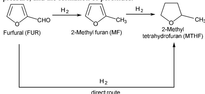
**Figure 19.** Different routes for the synthesis of 2-methyl tetrahydrofuran (MTHF) from furfural (FUR).
