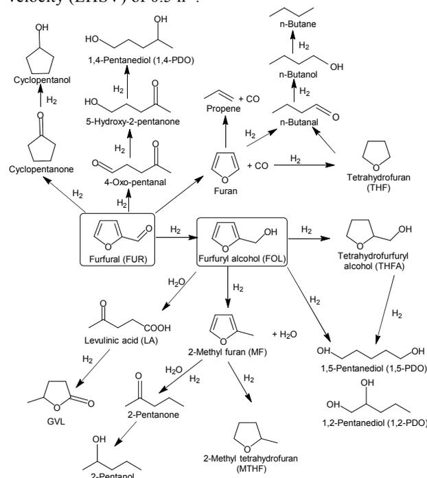
**Figure 5.** Various products formed during hydrogenation of furfural (FUR) to furfuryl alcohol (FOL).
