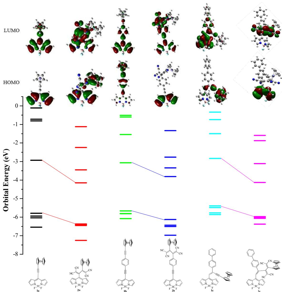
**Figure 3.** The comparison of frontier molecular orbitals and energy levels of BODIPYs **1a** – **1c** and **2a** – **2c**.
