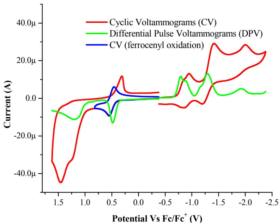
**Figure 2.** Overlaid Cyclic and differential pulse voltammograms (CV and DPV) of BODIPY **2b** recorded using glassy carbon as working electrode, Pt wire as the counter electrode, and saturated calomel electrode (SCE) as the reference electrode in  $\text{CH}_2\text{Cl}_2$  solvent and 0.1 M tetrabutylammonium hexafluorophosphate as supporting electrolyte.
